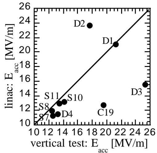
Fig. 2: Performance of the cavities after installation to the linac compared to the vertical test results.
