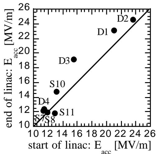
Fig. 4: Comparison of the cavity results obtained just after installation and after 3 months linac operation.
