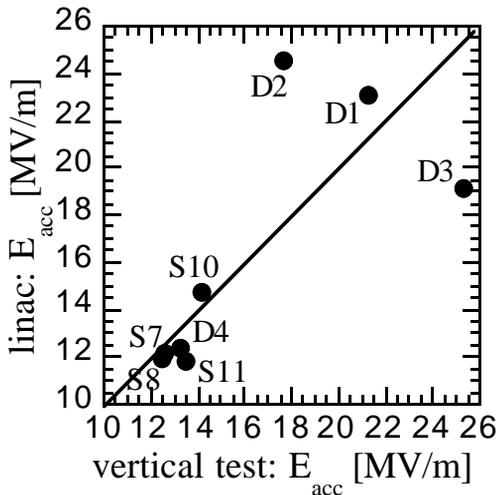
Fig. 3: Performance of the cavities after 3 months linac operation compared to the vertical test results.
