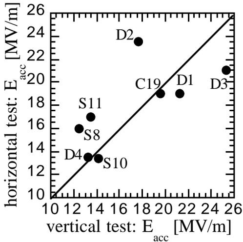
Fig. 1: Performance of the cavities in vertical and horizontal test.
