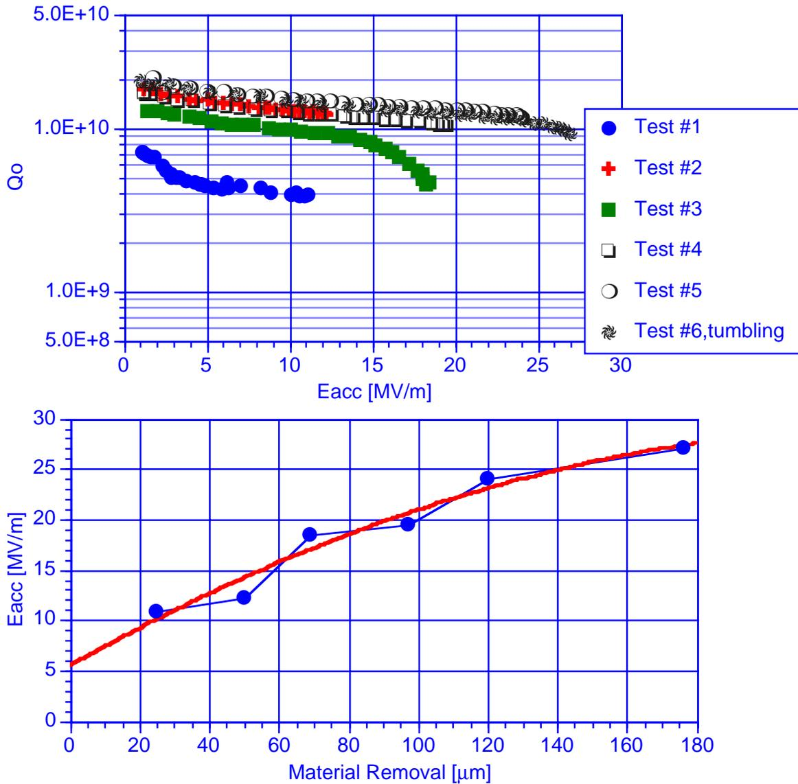
Figure 3: Dependence of achievable gradient on amount of material removal, measured on cavity K-17.
