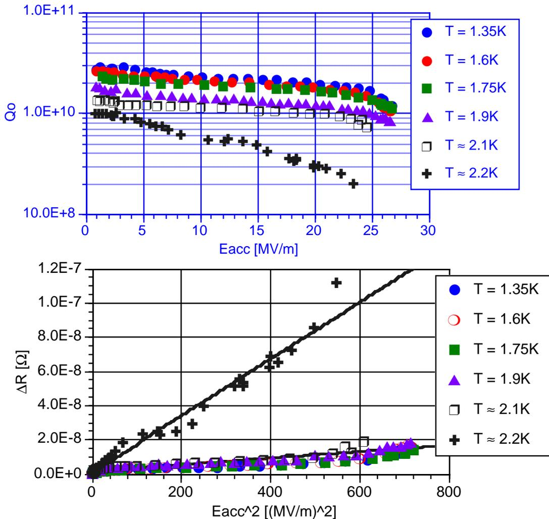
Figure 4: Results from tests on cavity JL-1. The slope in  $Q_0$  vs  $E_{\text{acc}}$  is caused by an additional resistance  $\Delta R \sim E_{\text{acc}}^2$ . The change in slope around  $T_\lambda$  points to a heat transfer problem at the defect.
