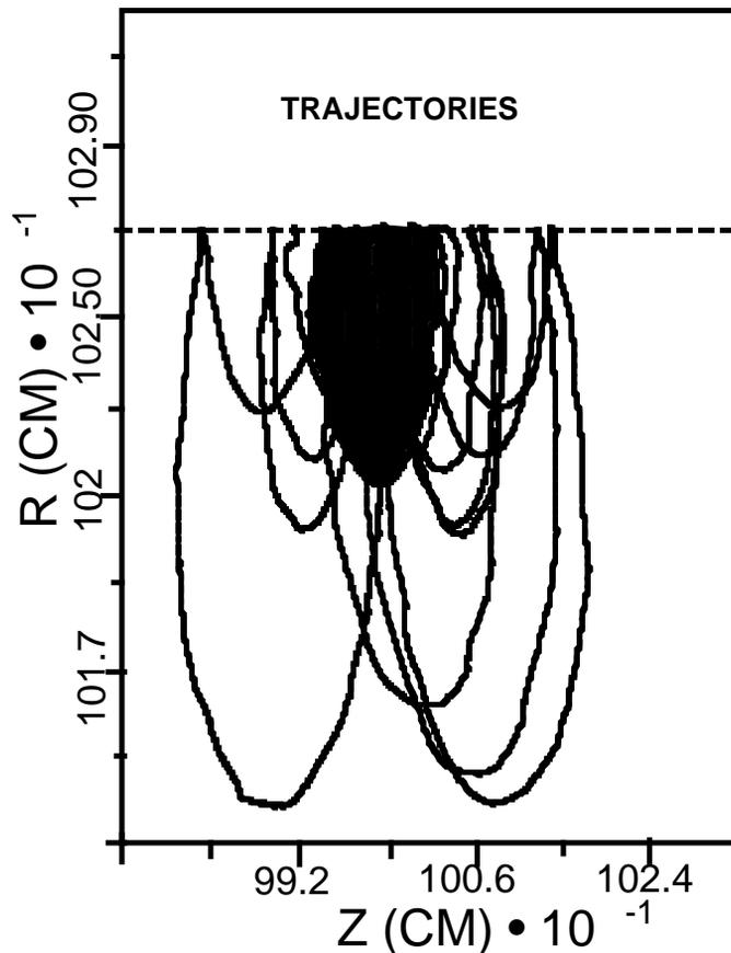
Figure 6: 2-point multipacting at  $E_{acc} \approx 25 \text{ MV/m}$ , corresponding to a peak magnetic field of  $H_{peak} \approx 1100 \text{ Gauss}$  at the equator of the cavity.
