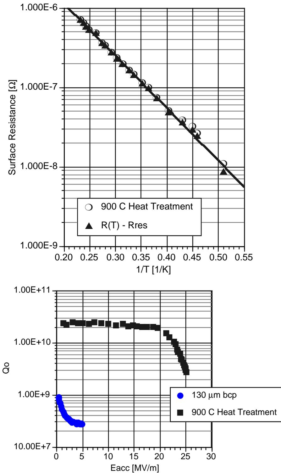
Figure 2: Performance of cavity K-16 . Strong Q-disease was seen immediately after barrel polishing and chemical treatment. After hydrogen degassing at 900° C a residual resistance of  $R_{RES}=2.2 \text{ n}\Omega$  was achieved and gradients up to  $E_{acc}=25\text{MV/m}$  were measured.
