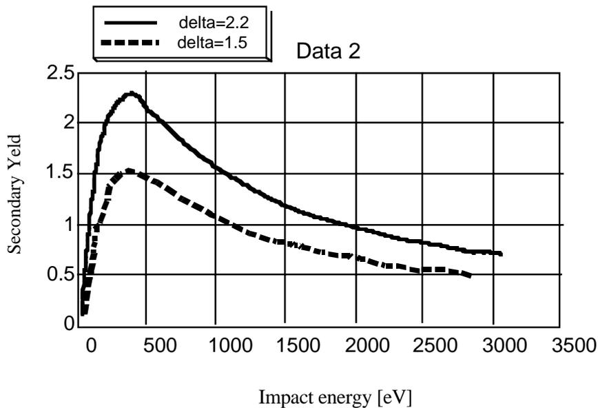
Figure 5: Secondary electron yield vs electron impact energy<sup>9</sup> used for the simulation calculations.
