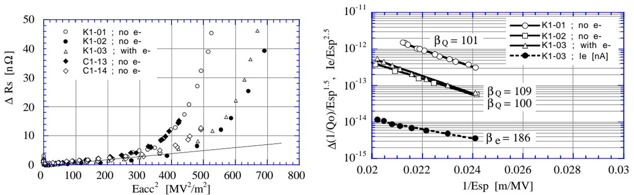
Figure 8. The increase of  $R_s$  with  $E_{acc}^2$ . Figure 9. The F-N plots of  $Q_o$  and  $I_e$ .
