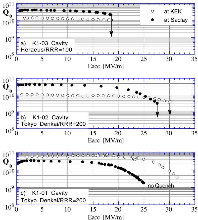
Figure 1. The  $Q_0$ - $E_{acc}$  curves in the KEK cavities tested at KEK and Saclay; a) K1-03 cavity, b) K1-02 cavity, c) K1-01 cavity.
