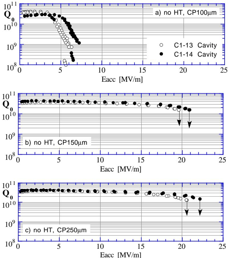
Figure 3. The  $Q_0$ - $E_{acc}$  curves in the Saclay/KEK collaboration cavities; a) no HT, CP100 $\mu$ m, b) no HT, CP150 $\mu$ m, c) no HT, CP250 $\mu$ m.
