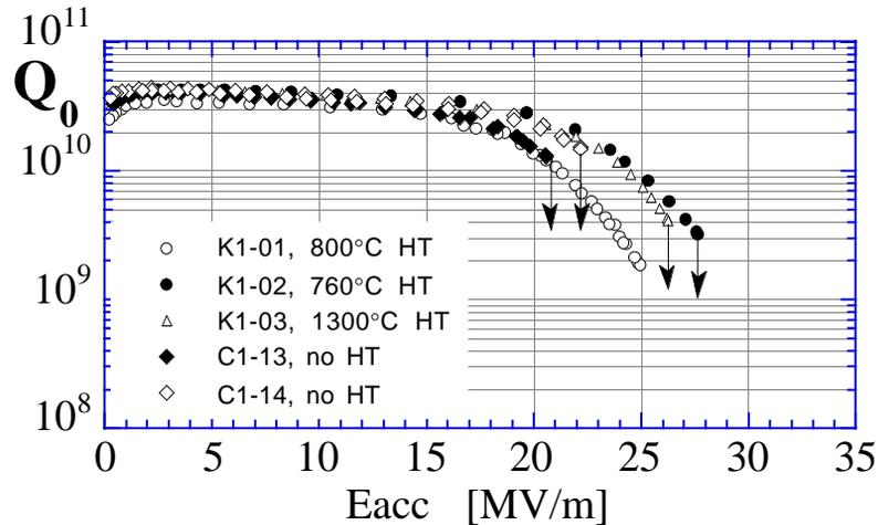
Figure 7. The Q<sub>0</sub>-E<sub>acc</sub> curves in the five cavities tested at Saclay.
