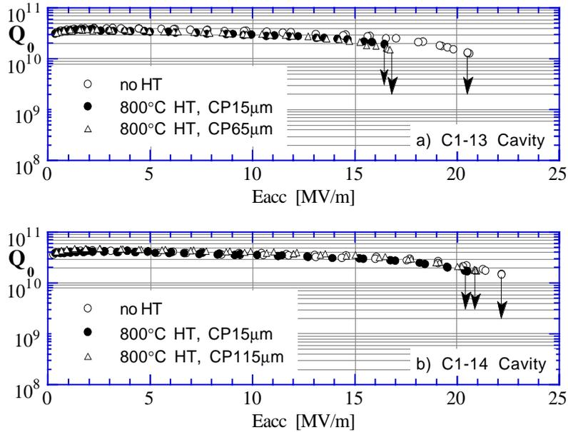
Figure 4. The  $Q_0$ -Eacc curves before/after 800°C HT; a) C1-13 cavity and b) C1-14 cavity.
