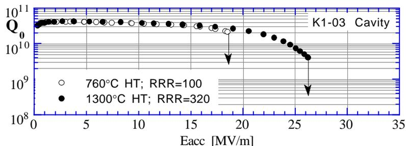
Figure 2. The effect of 1300°C HT at Saclay in the K1-03 cavity.
