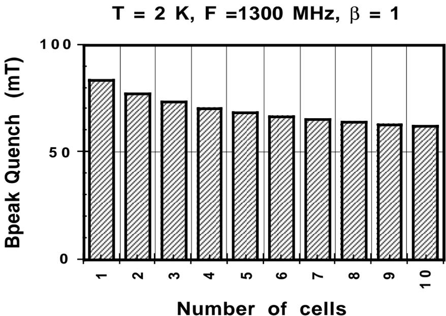
Figure 4 - The average quench field obtained decreases with the number of cells in a cavity as its surface increases. The quench field of a 9-cell cavity would be 25% lower when compared to a single-cell.
