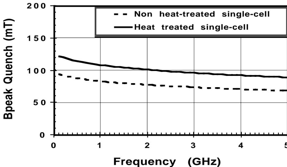
Figure 6 - Calculated quench field as a function of frequency taking in account both the thermal and the statistical analysis. The result show a rather low dependence on frequency, the two effects almost counterbalancing.
