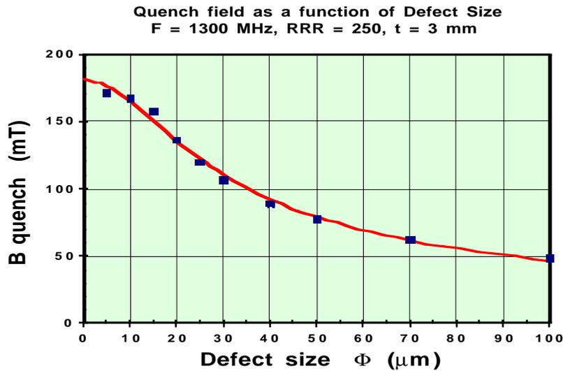
Figure 2 - The magnetic quench field decreases with the defect size. The points are calculated using thermal analysis. The line is the approximate expression used in this paper.
