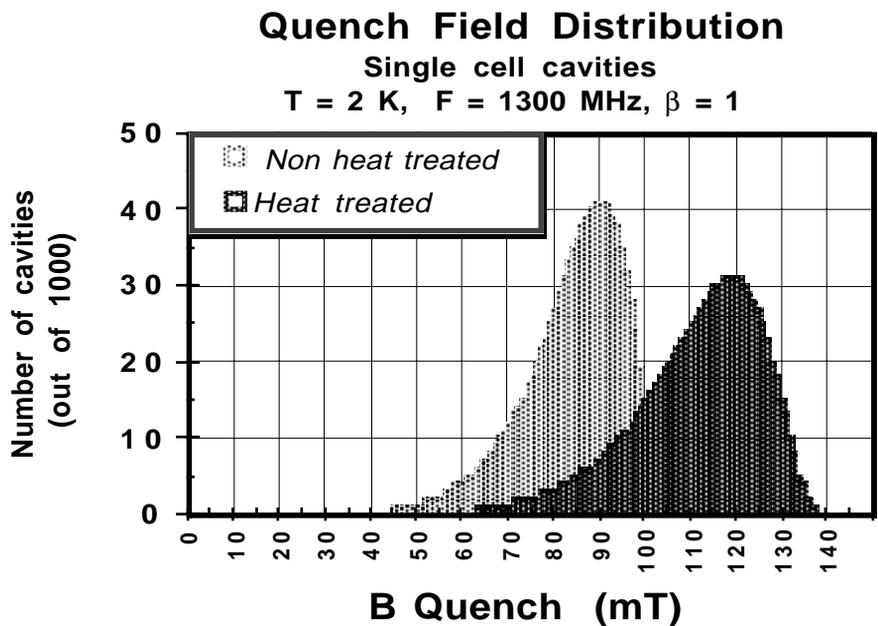
Figure 3 - Statistical calculated distributions of quench fields for non-heat treated and heat treated SCRF cavities.
