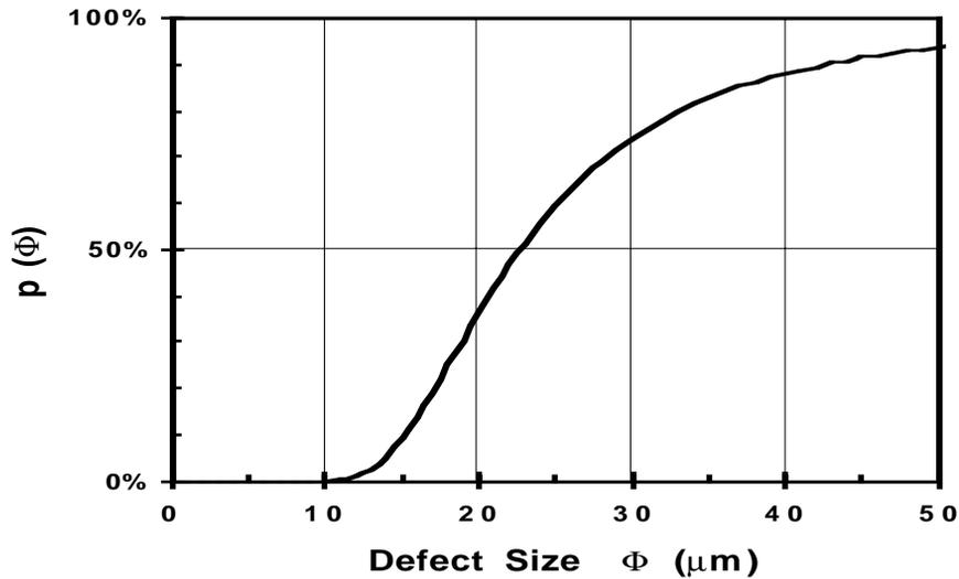
Figure 1 - Typical probability function variation with defect size.
