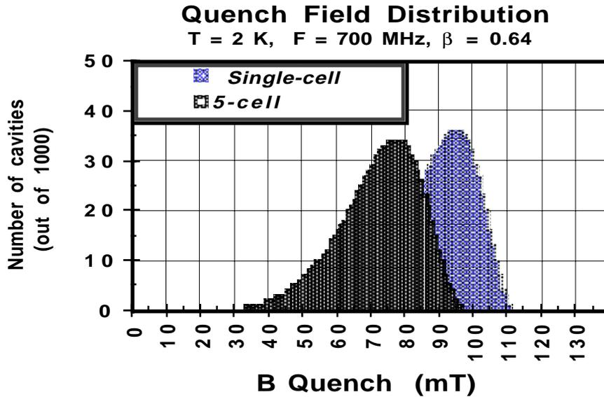
Figure 5 - Quench field distribution for non heat treated single and 5-cell proton cavities ( $\beta = 0.64$ ). The average expected quench field is slightly higher than for electron cavities at 1300 MHz.
