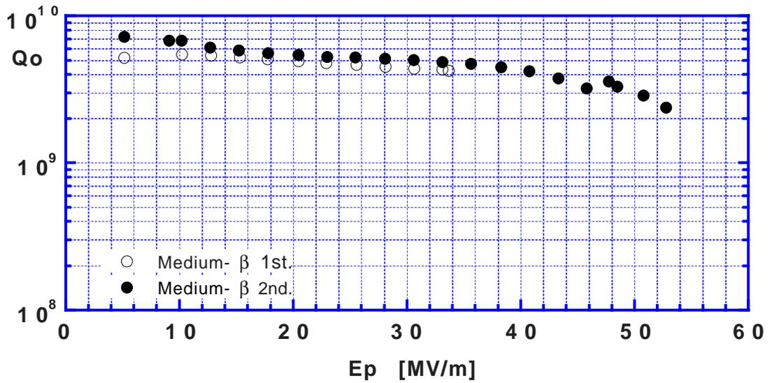
Fig. 3. Cold tested results on Qo-Ep curve.
