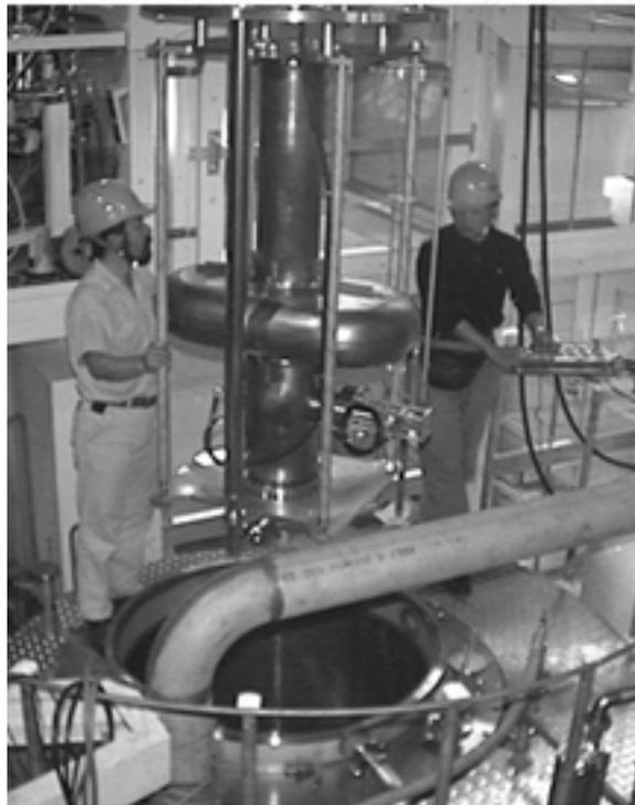
Fig. 6 KEKB crab cavity just before the installation into the virtual cryostat for cold test
