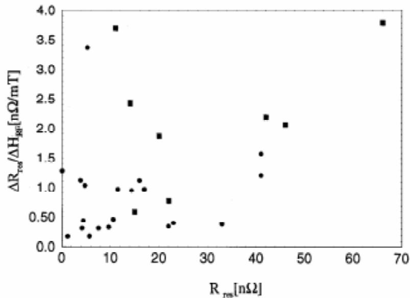
Fig. 16. Q-Slope versus residual resistance for Niobium sputtered Cu cavities. The round symbols refer to spun cavities, the square ones to hydroformed [34].
