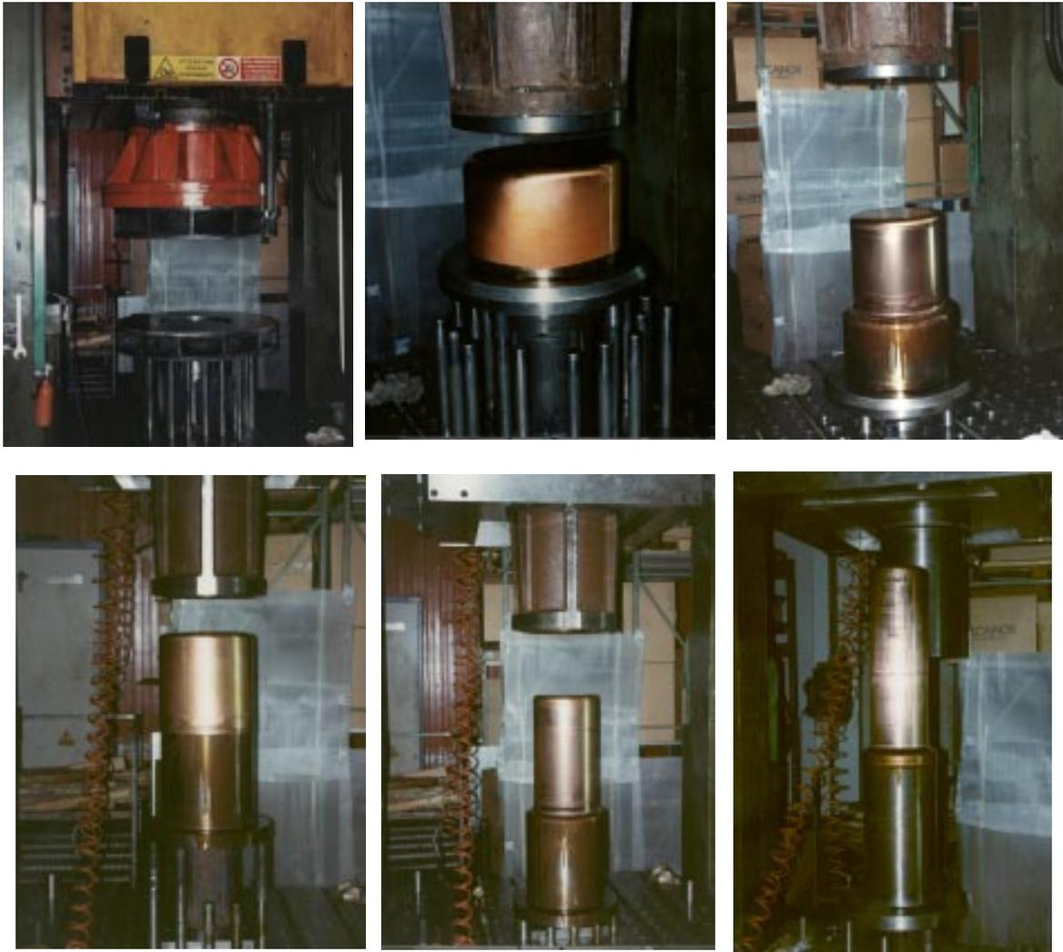
Fig. 20 First drawing and redrawing of the seamless copper tubes under investigation at LNL.
