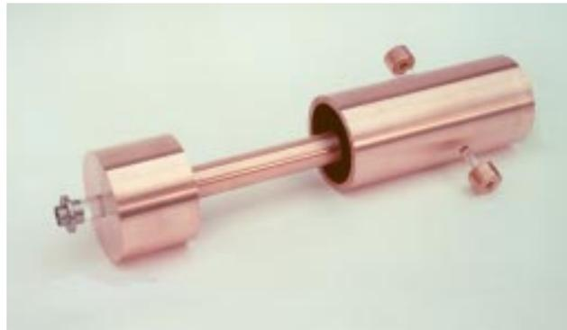
Fig. 23. The traditional fabrication way of a QWR. The resonator sizes are: 200 mm the external diameter, 80 mm the diameter of the central shaft, 600 mm the piece length.
