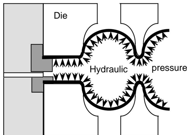
Fig. 5. Principle of Copper multicell hydroforming at CERN [15]
