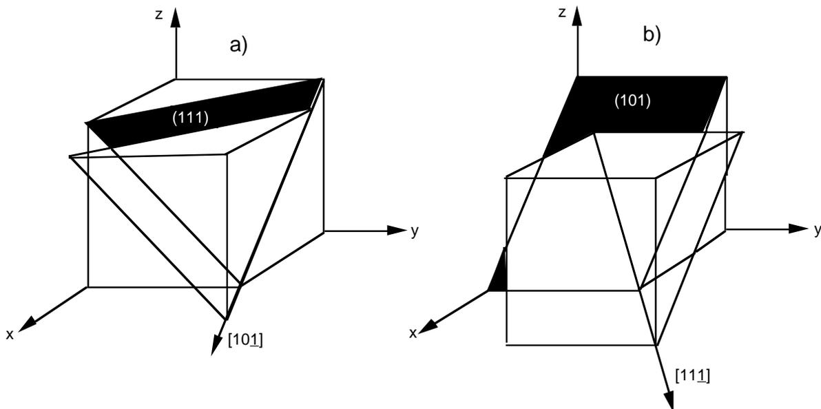
Fig. 3 a) Slipping system (111)  $[10\bar{1}]$  for FCC metals; b) slipping system (101)  $[\bar{1}11]$  for BCC metals. Among BCC metals, Niobium is a lucky exception since its anomalous slip direction  $[010]$  requires less energy for displacement if compared to the  $[\bar{1}11]$ .
