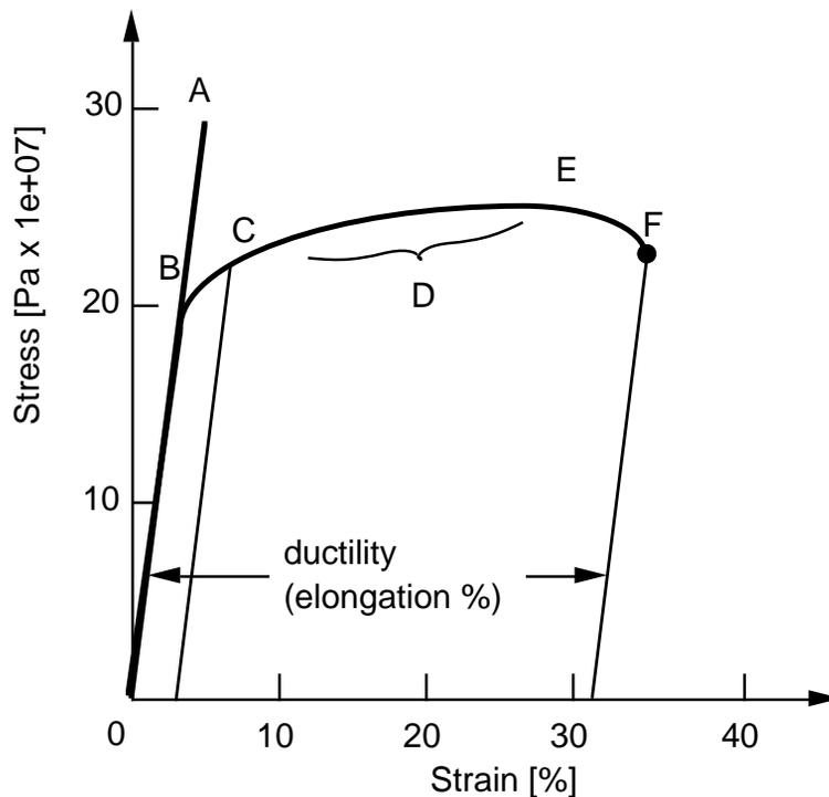
Fig. 1 A typical stress-strain curve for metallic materials
