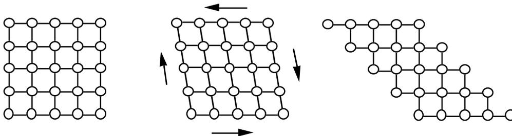
Fig. 2 Ideal model representation of plastic deformation of a crystal lattice by slipping, where all the atoms on both sides of the lattice planes are moved at the same time.
