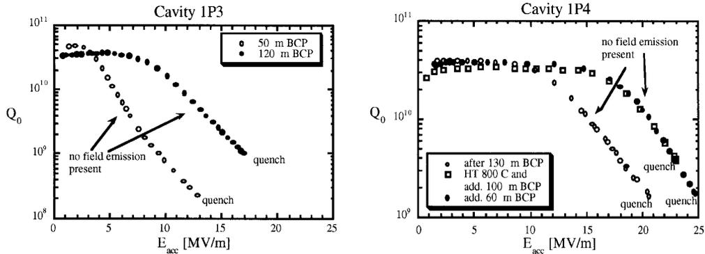
Fig. 14. Performances of first bulk Niobium 1.3 GHz monocells spun in LNL and characterized in DESY [46].
