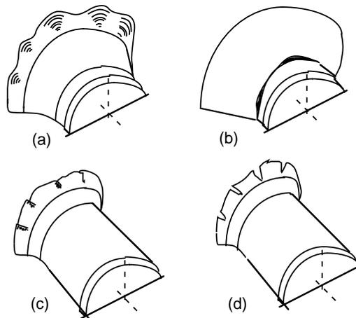
Fig. 9 Typical failures in spinning [12]: a) buckling due to tangential compressive strain; b) splitting due to radial tensile strain; c) splitting due to tangential compressive and bending strain; d) splitting due to tangential tensile strain after flipping the edge of the blank over.
