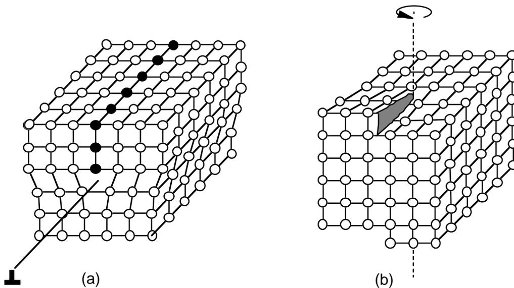
Fig. 4A dislocation can be split in two simpler components: a linear one (a), and a helicoidal one (b).
