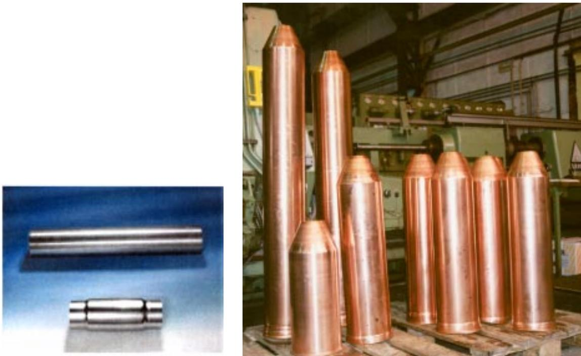
Fig. 22. Seamless tubes formed by flowturning: the Saclay Niobium tubes [courtesy C. Antoine] are on the left; the LNL flowturned Copper tubes are on the right.
