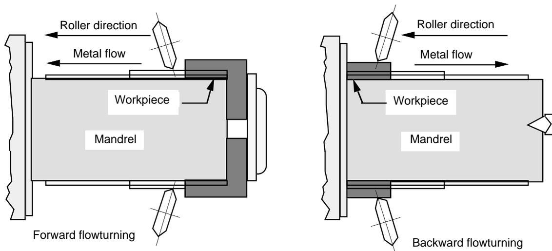
Fig. 21. Metal flow and roller travel in forward and backward flowturning.
