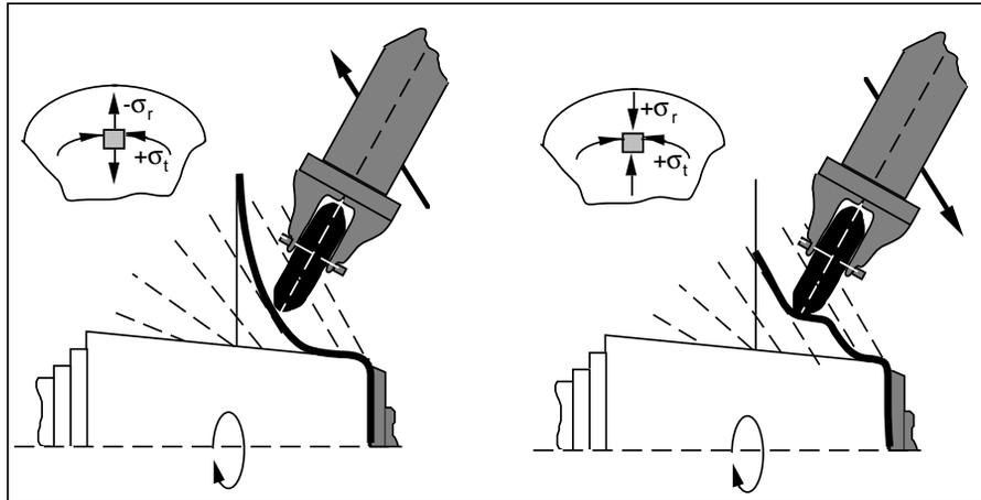
Fig. 8 Development of work zone and material stress during intermediate stages of spinning. The workpiece is shaped with a roller in several increments until the final shape is reached. A material element in the deformation zone is loaded by radial tensile and tangential compressive stresses. Let's define  $+\sigma_t$  = tangential stress,  $-\sigma_r$  = radial tensile stress,  $+\sigma_r$  = radial compressive stress.
