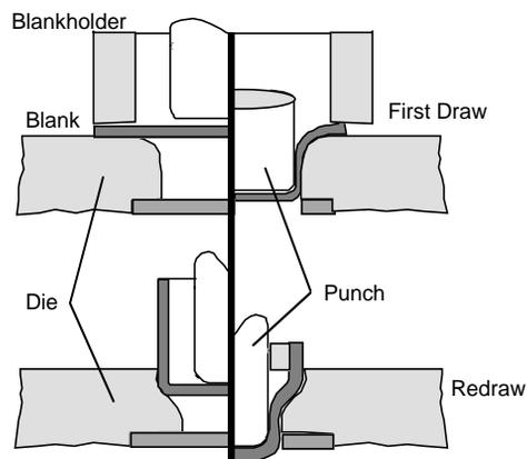
Fig. 18. Schematic diagram of the deep-drawing process with first draw (top) and first redraw (bottom), before starting the process (left) and during the process (right).
