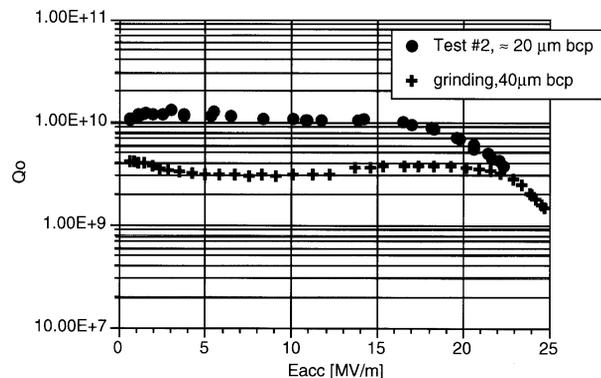
Fig. 15. Performance of a seamless 1.5 GHz cavity spun in LNL, sputtered at CERN and chemically processed and characterized in TJNAF [47].
