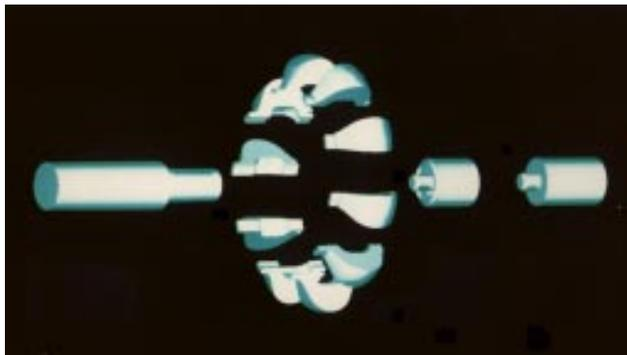
Fig. 13. Exploded view of the collapsible mandrel for 1.5 GHz cavities.
