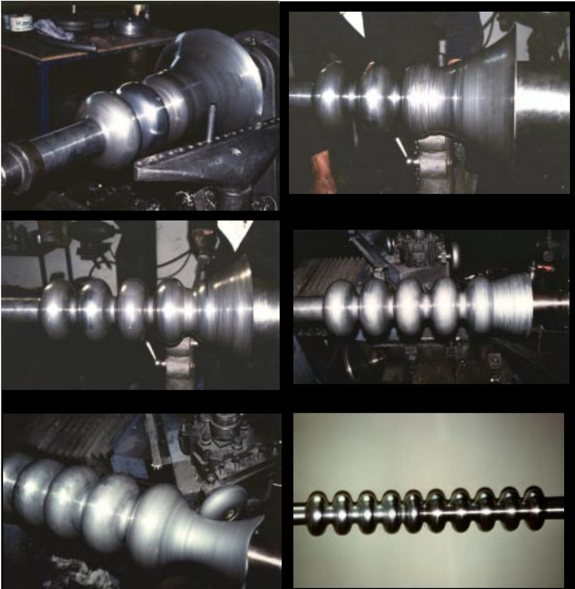
Fig. 12 Spinning of a 1.5 GHz Aluminum multicell prototype from a circular blank.
