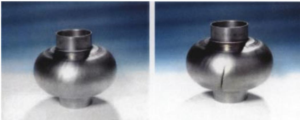
Fig. 6. Hydroforming tests performed at Saclay: rupture happened at 208% expansion instead of the 216% aimed [courtesy C. Antoine].
