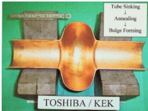
Fig. 7 Cut of a resonator formed by explosive bulging. The die consists of four sections, each divisible into half [courtesy K. Saito].
