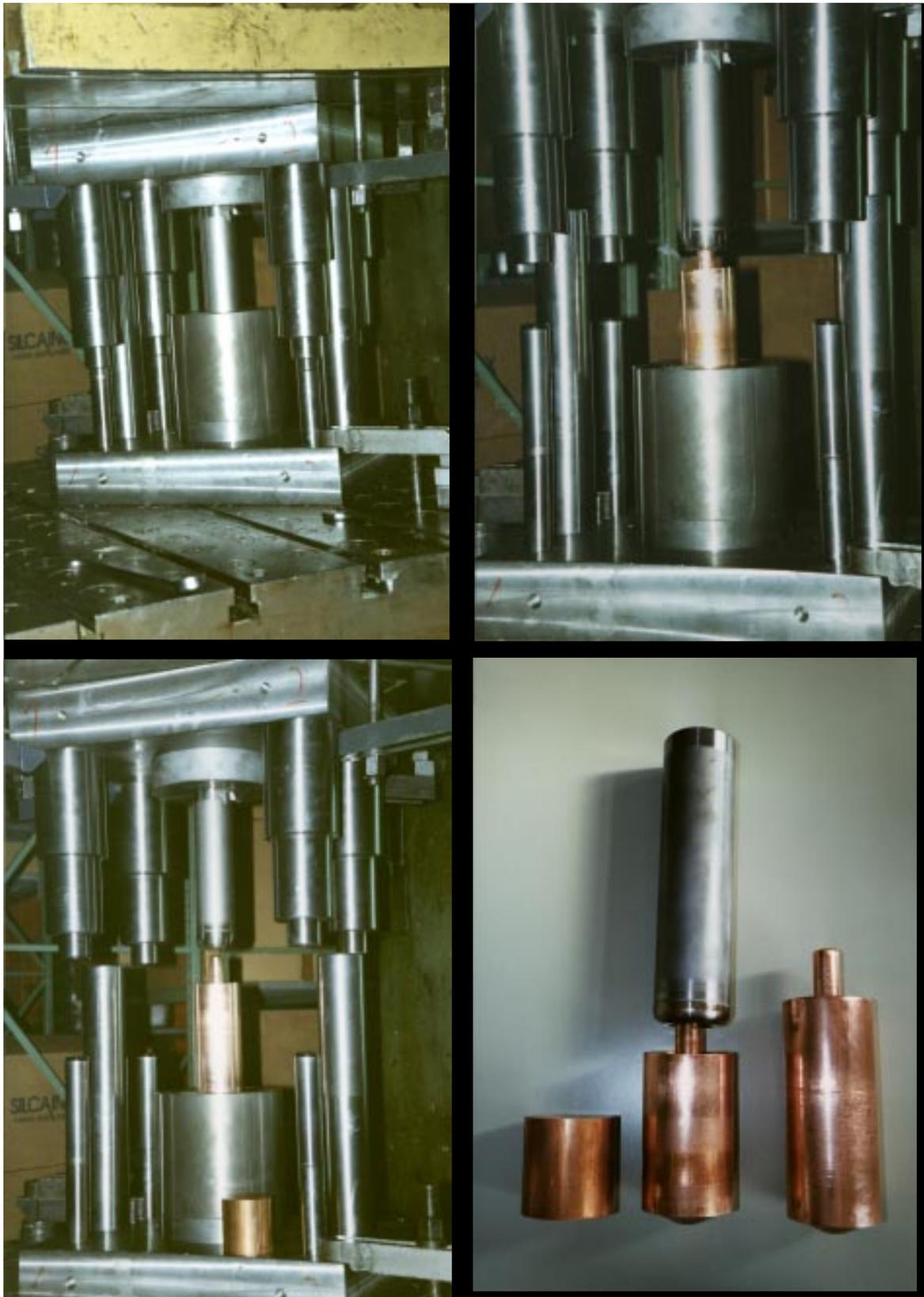
Fig. 24 Backward extrusion of a QWR 1:2.5 Copper model.
