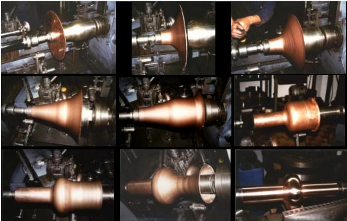
Fig. 11 Spinning of a 1.5 GHz copper multicell from a circular blank.
