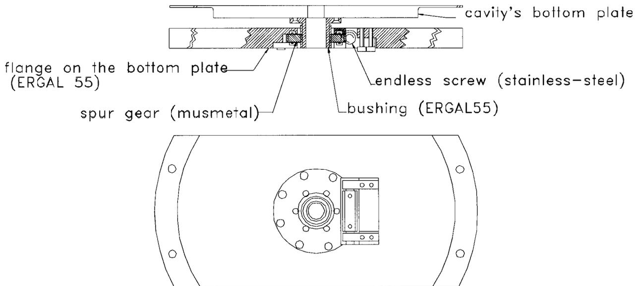
Fig 2: The fine tuning of the RFQ cavity is based on a bushing coupled through a spur gear to an endless screw which in turn is rotated by a stepping motor.
