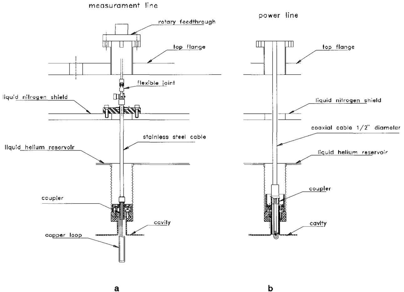
Fig 1: The measurement line (1a) used to multipactoring conditioning when the cavity is n.c. and to measure  $Q$  vs.  $E_a$  of the s.c. cavity. The power line (1b) used to overcouple and to control in operation the s.c. cavity with respect to a master oscillator.
