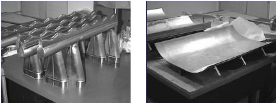
Fig.2: modulated electrodes with stems and stiffened tank quadrants, prepared independently, ready to be EB-Welded to one another
