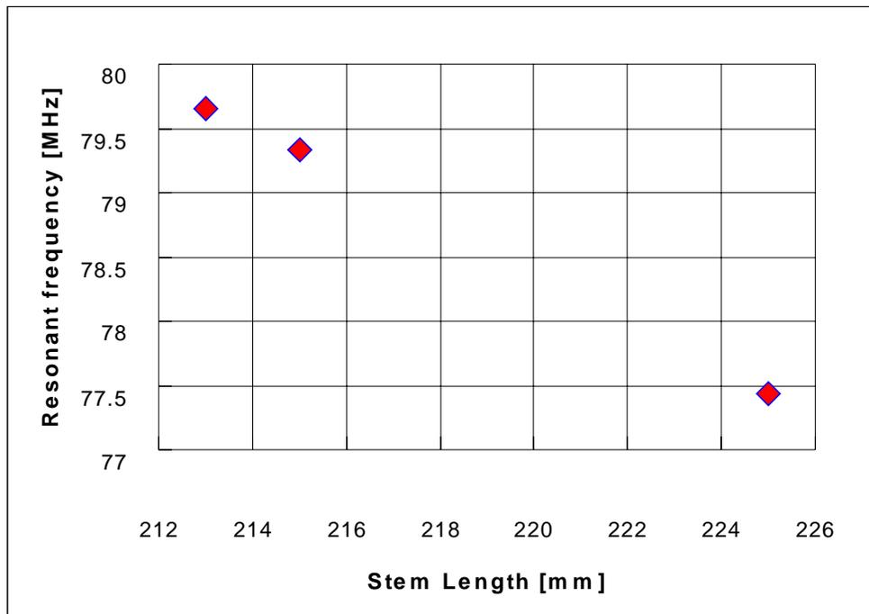
Fig.4: The result of the rough tuning frequency measurements is shown. The frequency sensitivity to the length reduction of the stems is  $\Delta f/\Delta l \sim 180$  kHz/mm. Taking thermal shrinkage (from 300 to 4 K) into account, and the consequent frequency increase, the target frequency is  $f_0 = 79.75$  MHz at room temperature for stainless steel.
