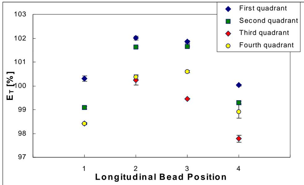
Fig.5: . Bead measurements in the four quadrants of SRFQ2: field bumps are within  $\pm 2\%$ . The positioning of the electrodes, when the measurements were taken, was with  $\pm 0.3$  mm with respect to the nominal position. Positioning was better after completion of the construction and the final welds.
