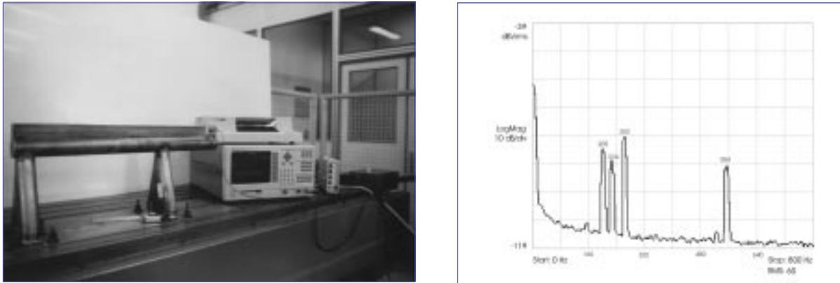
Fig. 6: experimental setup and frequency spectrum of the mechanical eigenmodes of the single electrode. The experimental values of the two lowest eigenmodes are lower than the estimated ones, by 8% and 25% respectively.
