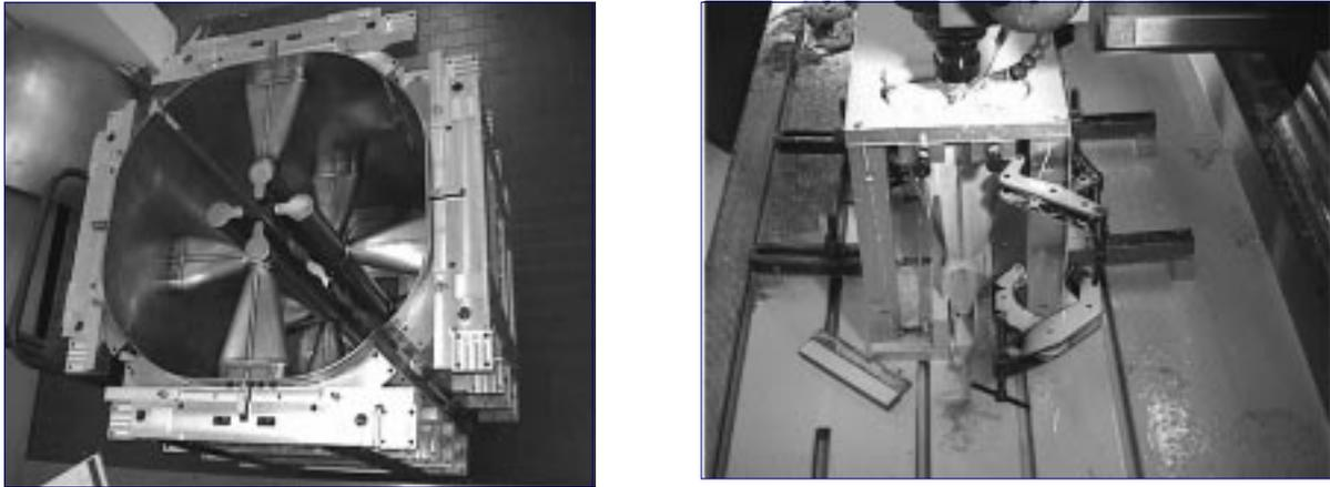
Fig.3: The stainless steel RFQ prototype being assembled in its jig for the first frequency measurement (first image) and one of the stems being cut by milling machine in order to squeeze the cavity and increase the frequency in the following measurement (second image).
