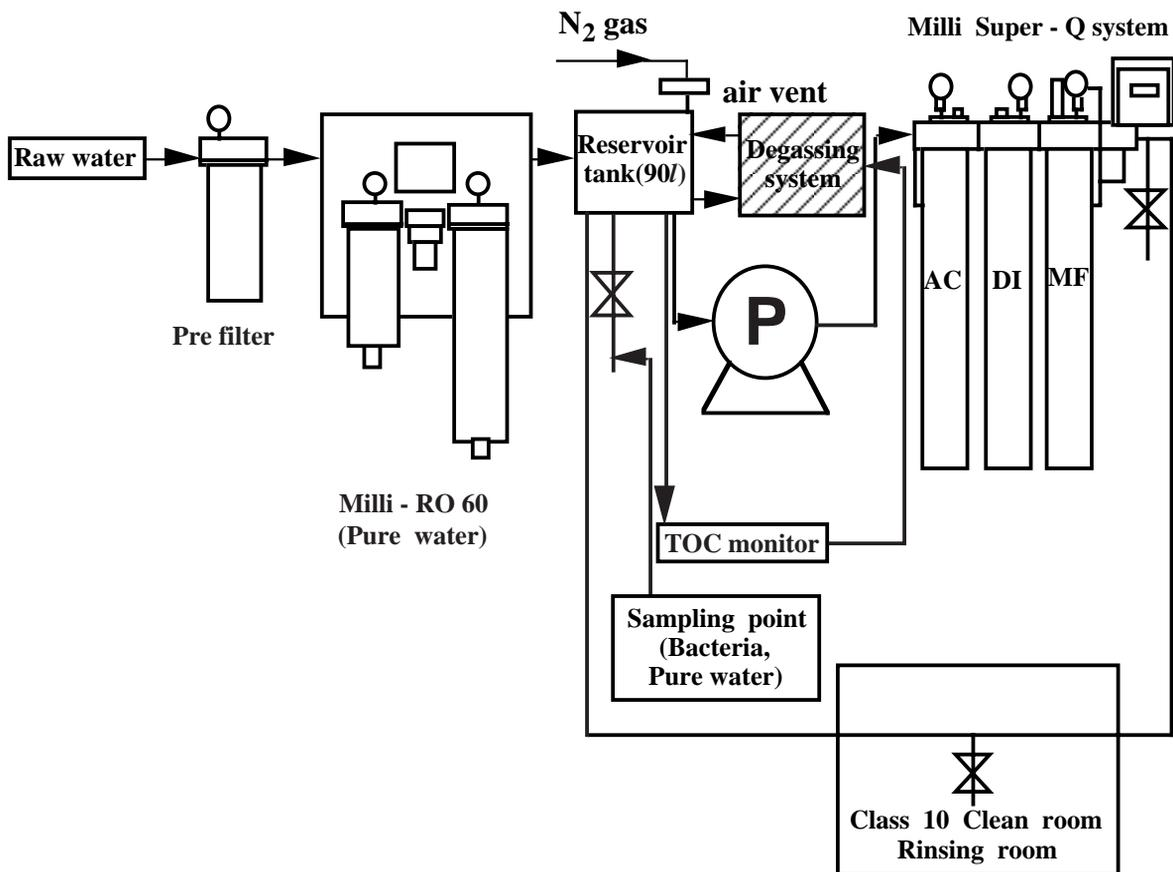
**Fig. 2. Experimental set up.**
