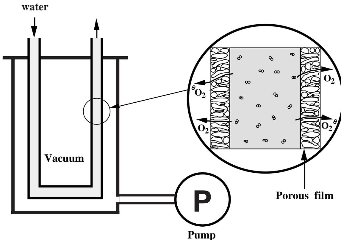
Fig. 1. Principle of degassing of water.
