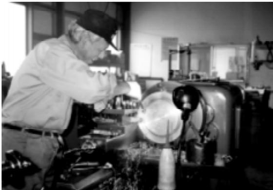
Fig. 1: Trimming of a half cell
