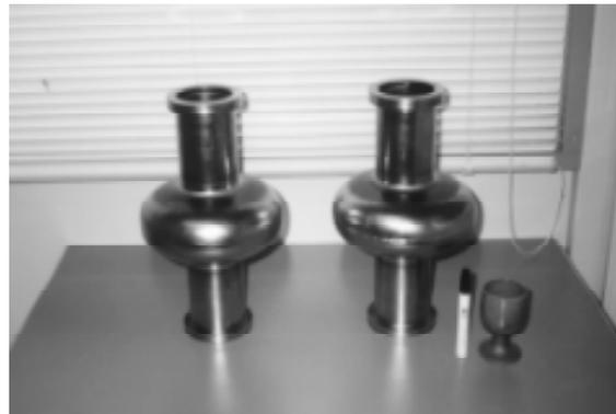
Fig. 2: Two niobium cavities
