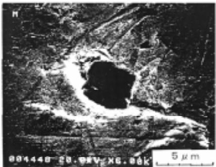
SEM image and size of an embedded abrasive (× 6000)
