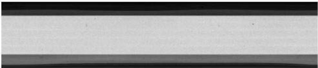
Figure 13 : (a) Echo images of the absorber with 3 mm-thick soft steel layer over copper before baking (#11S2). (b) After baking at 150 °C.
