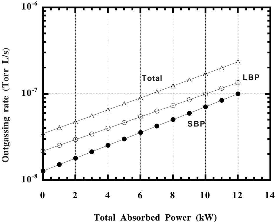
Figure 5 : Calculated outgassing rate as a function of total absorbed power using experimental data.
