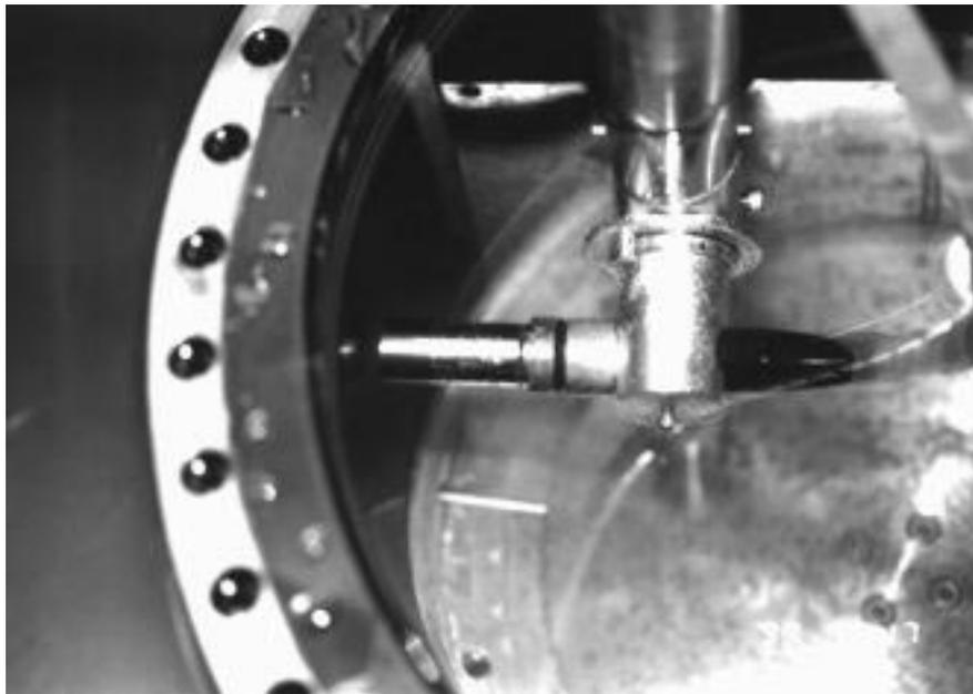
Figure 8 : Apparatus for acoustic tomography when a HOM absorber is being measured.
