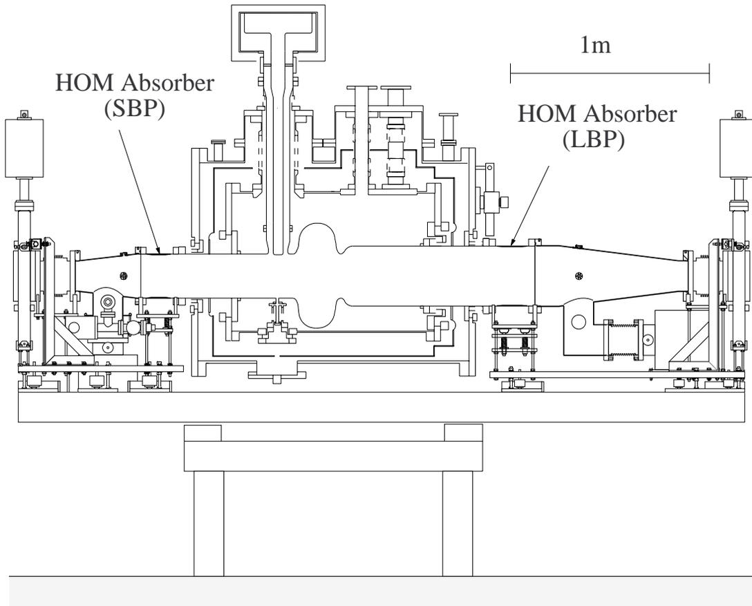
Figure 1 : Superconducting cavity module for KEKB.
