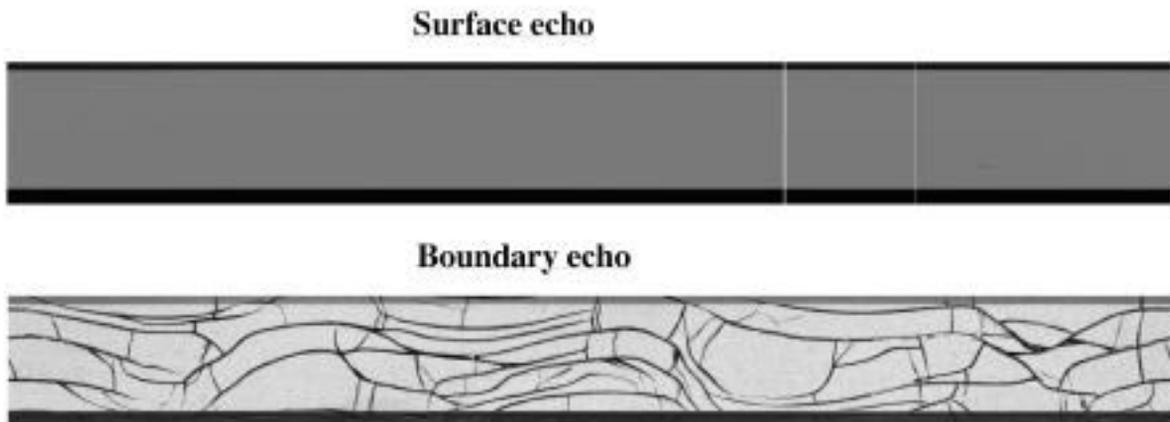
Figure 10 : Images of echoes from ferrite surface and copper/ferrite boundary. This absorber (#6S3) was used for beam tests in TRISTAN AR. Cracks are clearly seen in the boundary echo. Widths of cracks were less than 10  $\mu\text{m}$  and too narrow to be detected by the surface echo.
