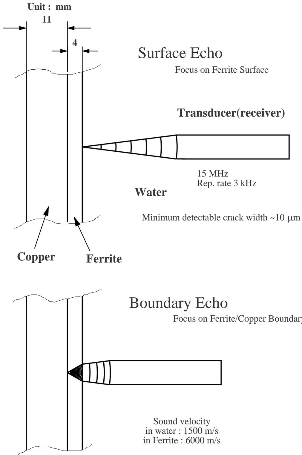
Figure 7 : Schematic of acoustic tomography. Measurements of the echo from the ferrite surface and that from the boundary between ferrite and copper.
