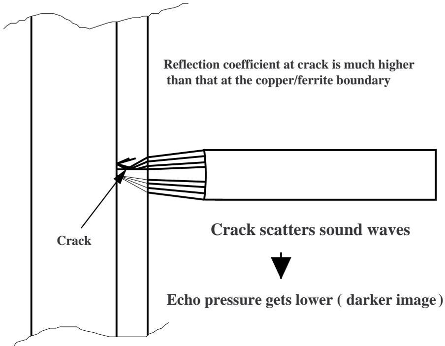
**If a crack is in parallel with the surface, i.e. delamination,**
