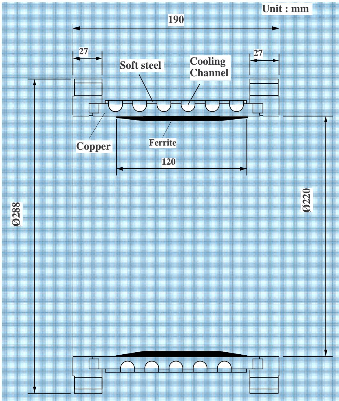
Figure 14 : Modified design of the absorber (Small Beam Pipe). The ferrite thickness is 4 mm with 25 mm long tapers at both ends. 3 mm-thick soft steel layer is left on copper.
