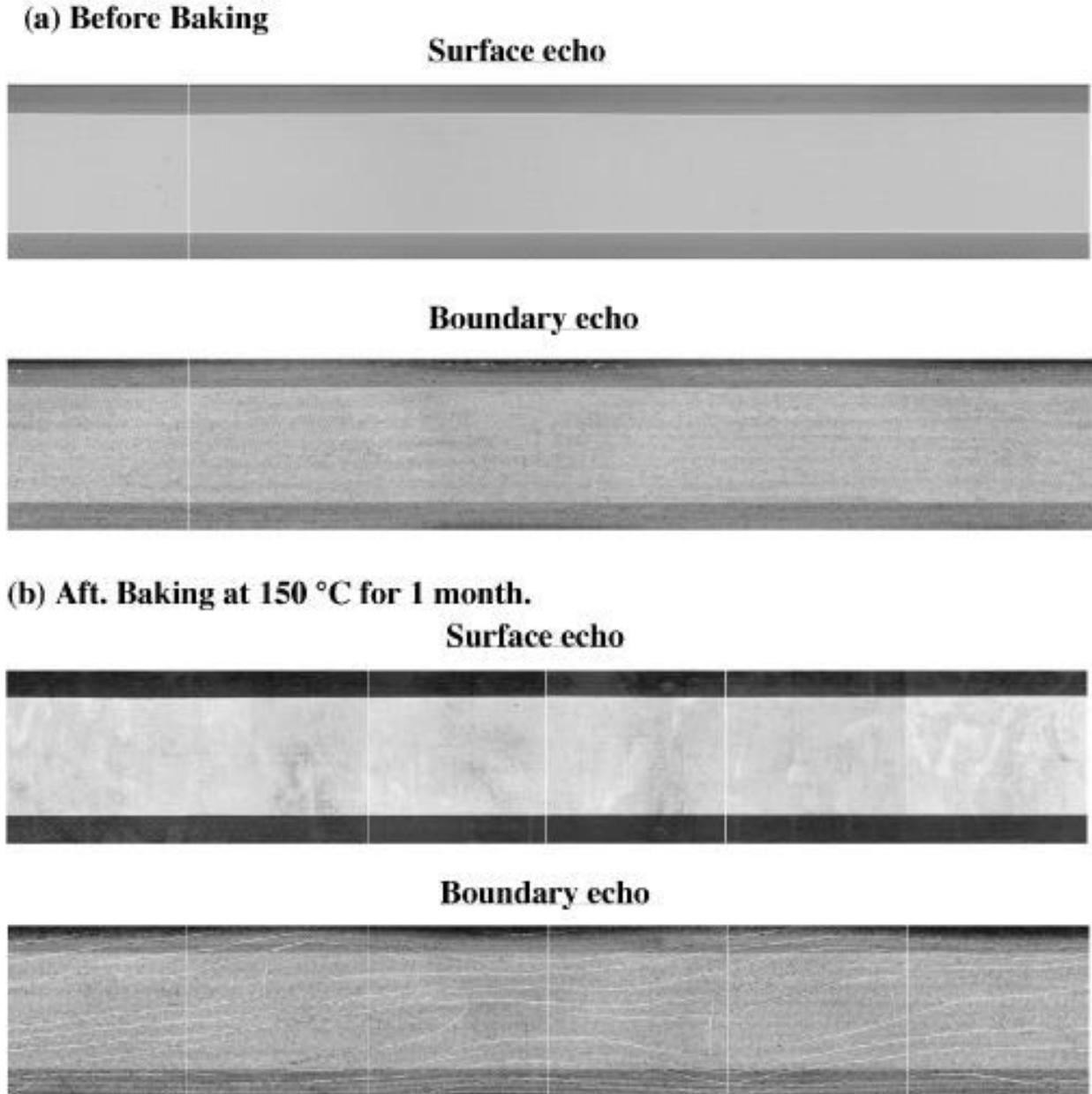
Figure 11 : (a) Echo images of the absorber before baking (#7LA). (b) After baking at 150 °C for 1 month.
