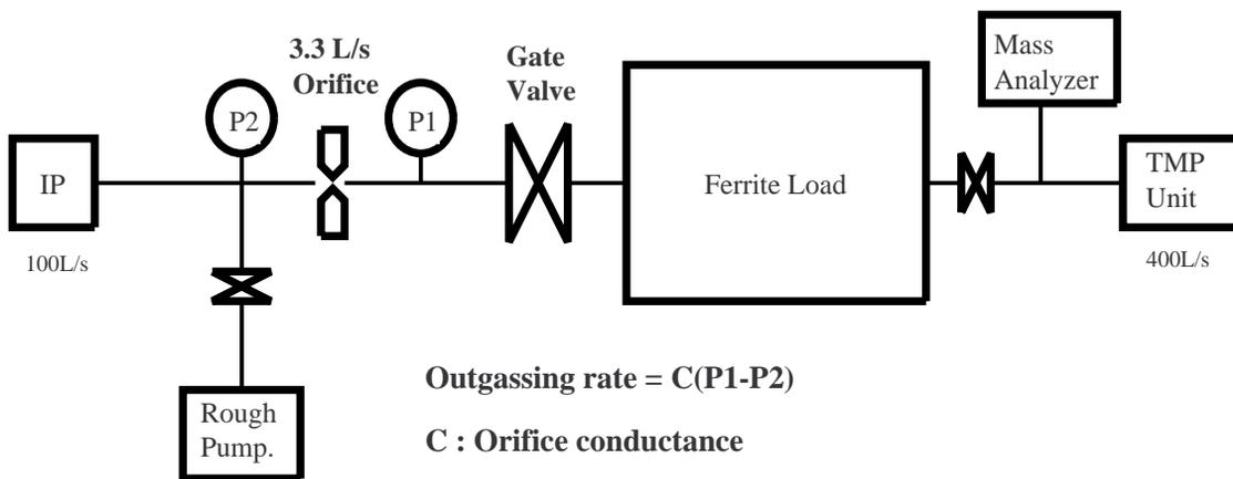
Figure 3 : Schematic of outgas measurement setup.
