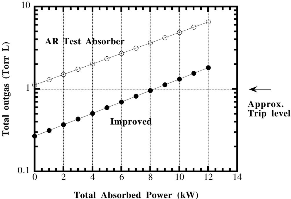
Figure 6 : Total amount of gas after 3 months of operation as a function of total absorbed power.
