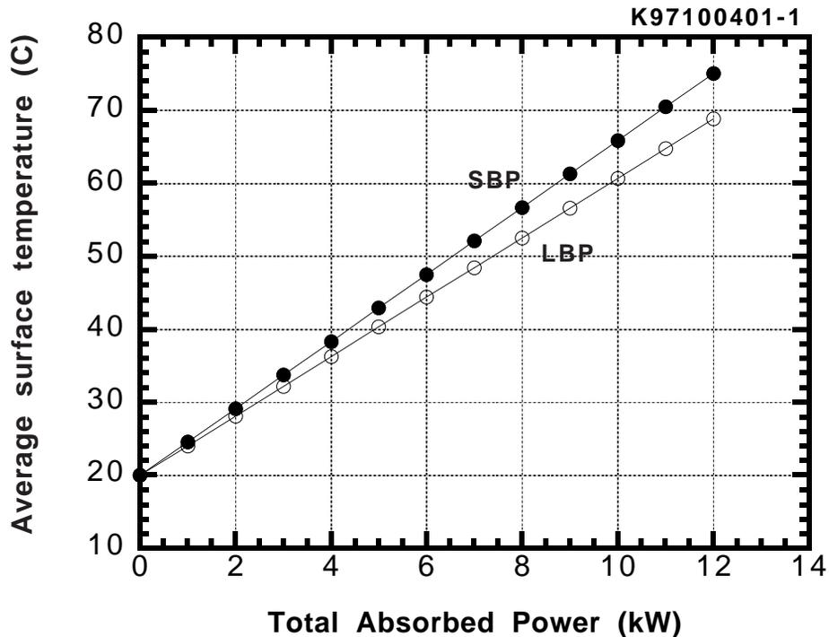
Figure 2 : Calculated average surface temperature of ferrite as a function of total absorbed power.
