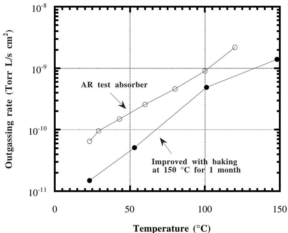
Figure 4 : Outgassing rate as a function of temperature. Reduction of outgassing rate with further baking can be seen.
