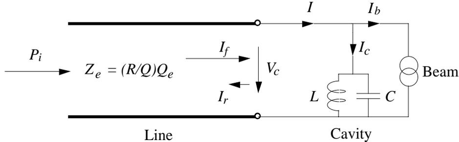
figure 2: Simplified circuit diagram of beam loading
