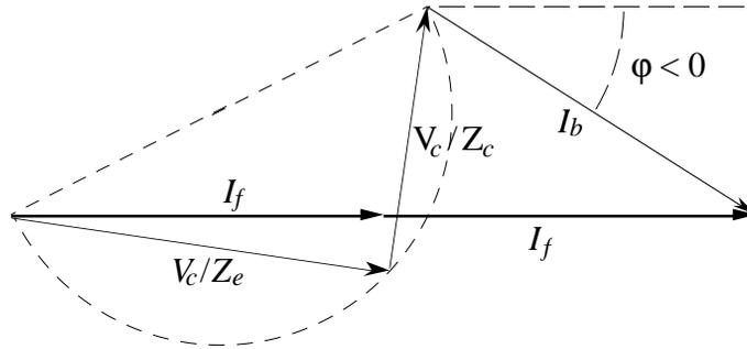
Figure 3: Phasor diagram of beam loading
