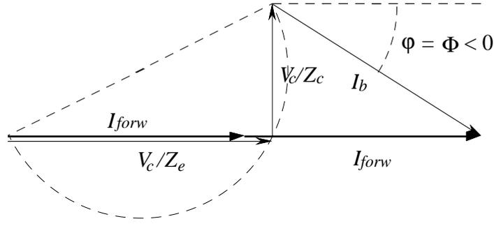
Figure 4: Phasor diagram for optimal detuning
