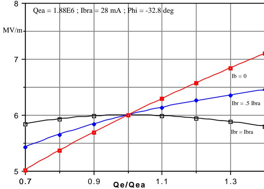
Figure 5: Coupling dependence of the acc. gradient for three different beam currents
