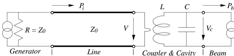
Figure 1: The basic elements of an accelerating station.
