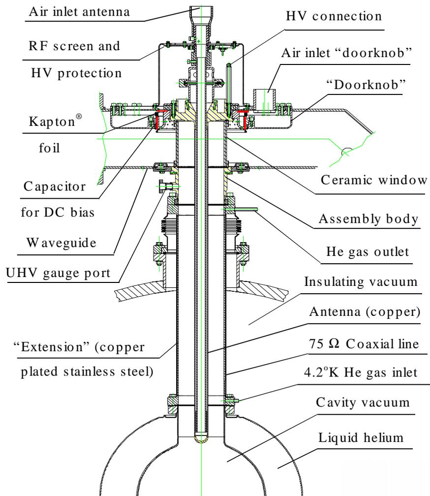
**Figure 1** Layout of the 75 Ω fixed coupler for LEP2
