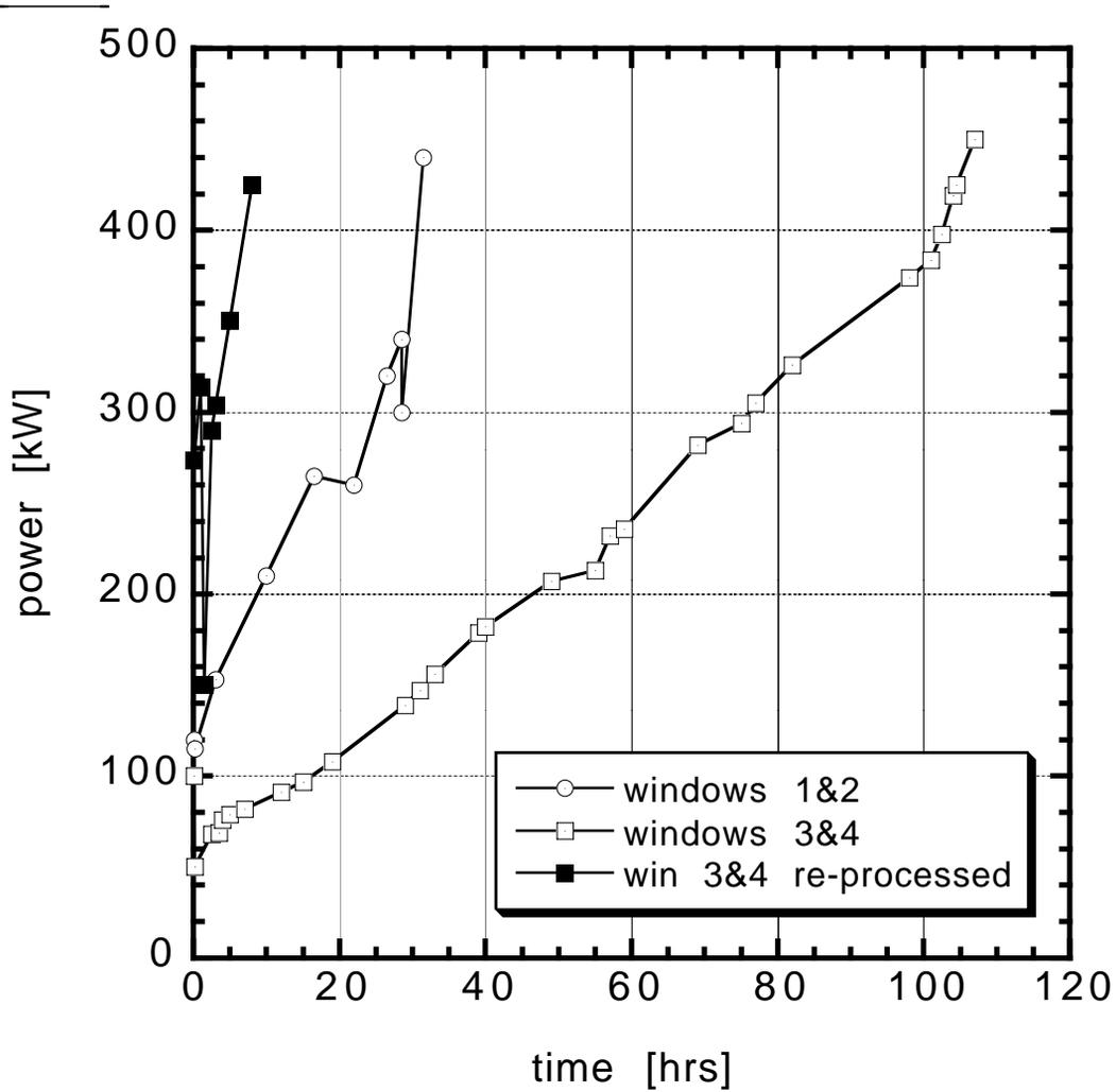
Figure 3. RF power propagated vs. time for processing of two window pairs. In addition to initial processing, also plotted is the case for window pair 3&4 being let up to atmospheric pressure of clean nitrogen gas, pumped out, and reprocessed. For window pair 1&2, power levels plotted above 300 kW are peak power with a 33% duty cycle.
