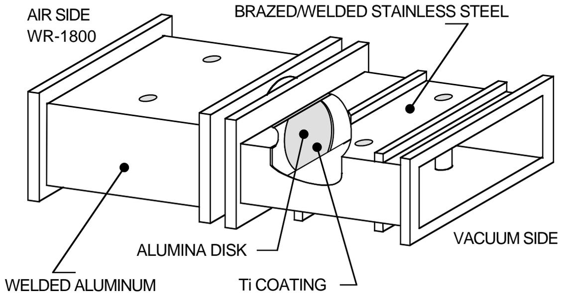
Figure 1. Schematic of a Thomson waveguide window.
