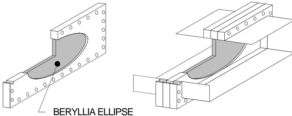
**Figure 5.** Illustration of a self-matched window utilizing an elliptical beryllia ceramic of uniform thickness in reduced-height waveguide. On the left is the window assembly alone and on the right is the window connected to waveguide.
