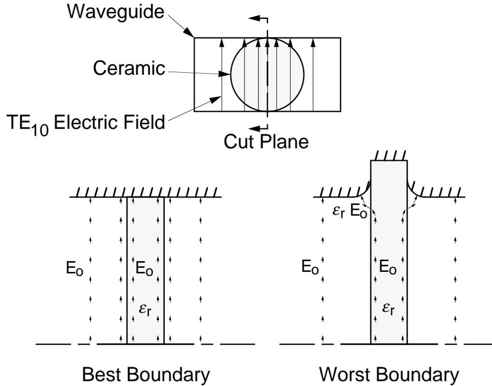
**Figure 6.** Conceptual illustration of a fictitious ceramic window with cross sections showing the ceramic-metal-vacuum boundary, so-called triple point. Electric field vectors are indicated in the bottom part of the figure with lengths illustratively proportional to field amplitude.
