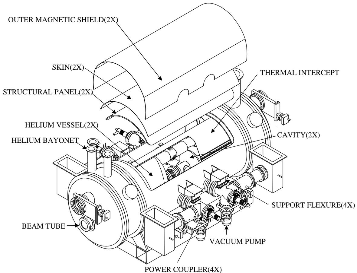
Figure 1.  $\beta=0.64$  Cryomodule with the thermal intercept and helium vessel cut away.
