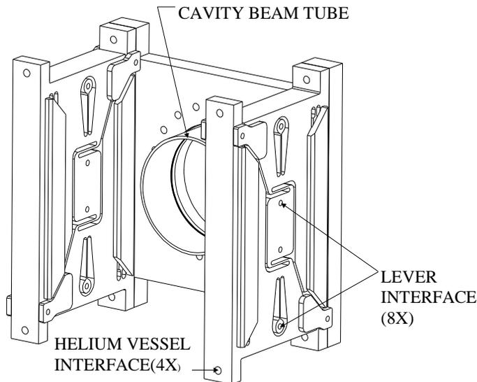
Figure 3. Cavity frequency tuner
