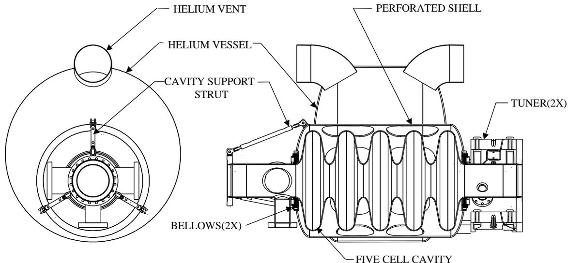
Figure 2.  $\beta=0.64$  cavity and helium vessel assembly
