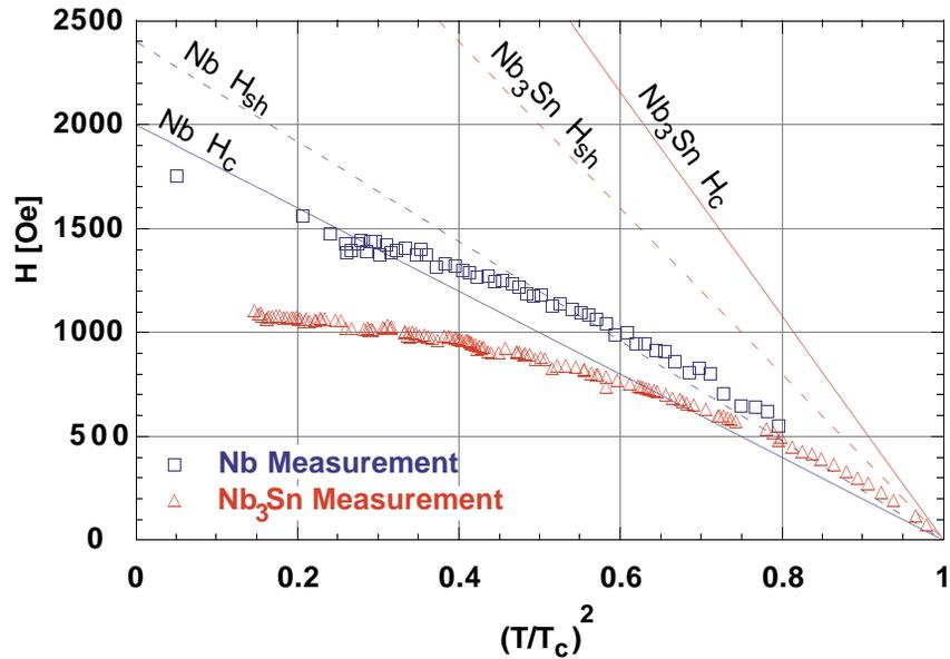
Figure 6: Comparing the niobium and Nb<sub>3</sub>Sn measurements against the superheating critical field predictions.
