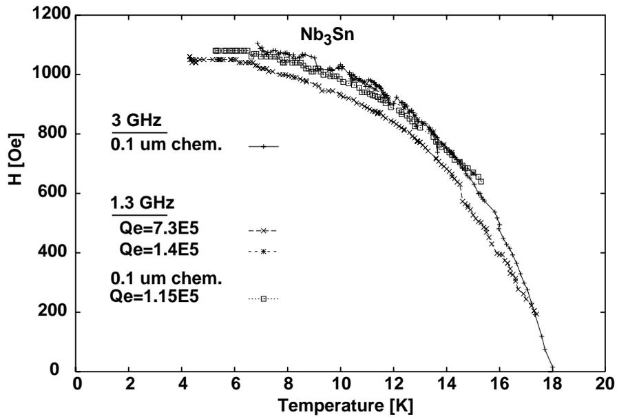
Figure 5: Measuring the  $H_c^{rf}$  of  $Nb_3Sn$  by pulsing a  $Nb_3Sn$  coated niobium 1.3 GHz cavity and a  $Nb_3Sn$  coated niobium 3 GHz cavity. Multiple measurements were made on the 1.3 GHz cavity with different couplings and surface treatment.
