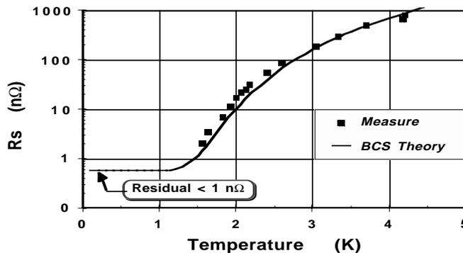
Figure 7 - Surface resistance measured on a single-cell cavity at a frequency of 1300 MHz and an accelerating field of 0.5 MV/m. The theoretical fit is obtained with the BCS theory and a residual resistance of 0.57 n $\Omega$ .
