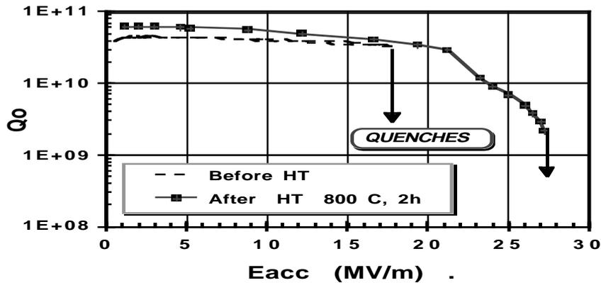
Figure 5 - The cavity C110 made from niobium RRR 400 sheets improved its quench field after only a 800°C, 2 hours annealing.
