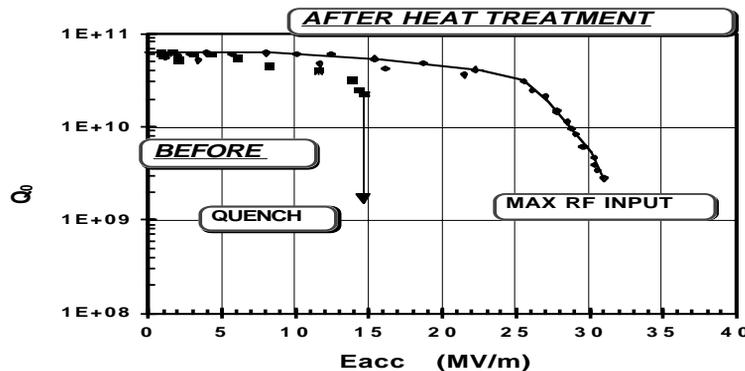
Figure 4 - Single-cell cavity C101 (initial RRR 250), quenching at 15 MV/m before heat treatment. The improvement after heat treatment is impressive ( $> 31\text{ MV/m}$  without quench).
