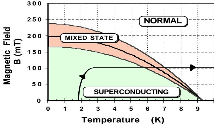
Figure 1 - Phase diagram of niobium giving the critical magnetic fields ( $B_{c1}$ ,  $B_c$ ,  $B_{c2}$ ) as a function of temperature.
