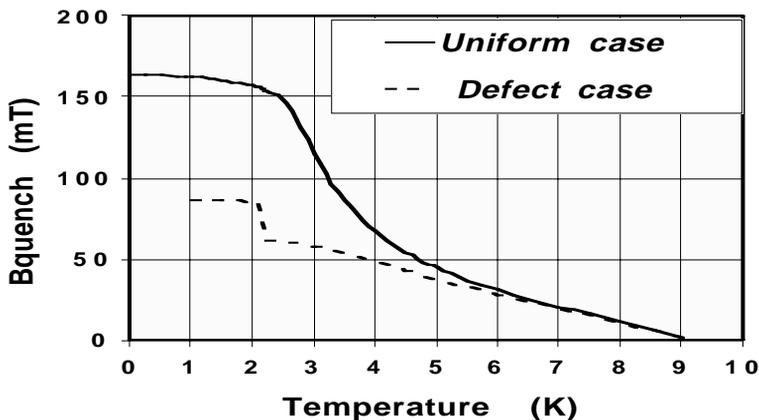
Figure 2 - Calculated quench field value for a niobium RRR 200 cavity, thickness 2.5 mm at a frequency of 1300 MHz in the uniform case and in the case of a normal defect (size = 20  $\mu\text{m}$ ,  $\sigma = 10^7 \Omega^{-1} \cdot \text{m}^{-1}$ ).
