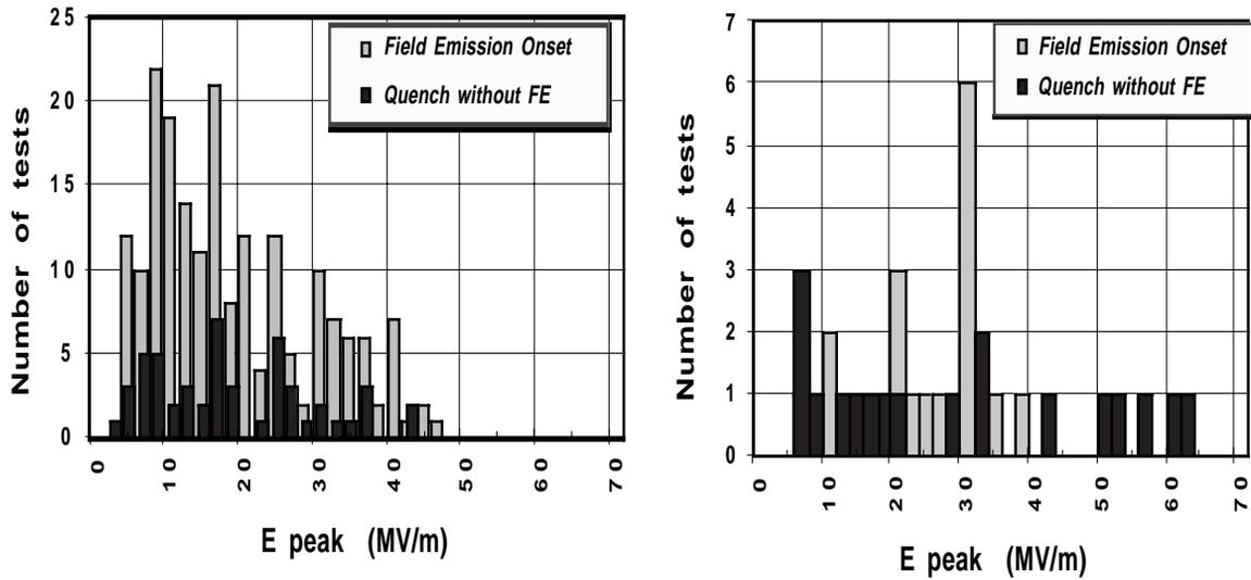
Figures 6a & 6b- Field emission thresholds statistics on 320 tests performed at Saclay before and after January 1996. Cavities without FE are now obtained with peak fields exceeding 60 MV/m.
