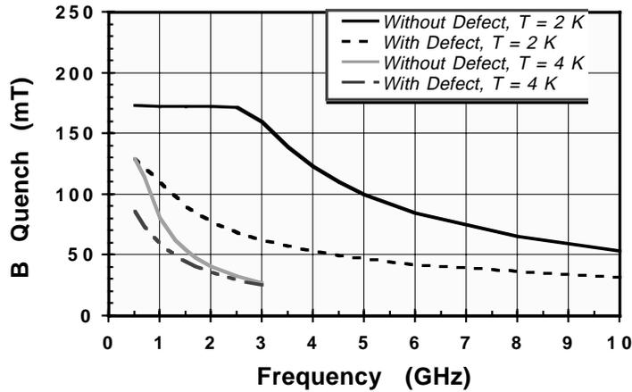
Figure 3 - Calculated quench field value with and without defect as a function of frequency for a RRR 250 niobium cavity and helium bath in the superfluid state ( $T = 2\text{ K}$ ) and normal state ( $T = 4\text{ K}$ ).
