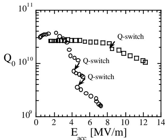
Fig. 3: Excitation curves of cavities with localized strong defects in the bulk material. So called "Q-switches", stepwise degradation of quality factor with increasing incident power, are observed.
