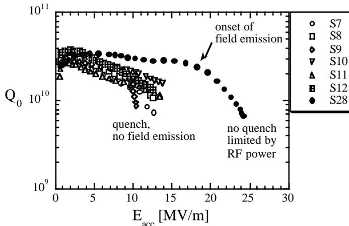
Fig. 4: RF-performance of cavities produced by one manufacturer with old (S7 to S12) and improved (S28) welding technique.
