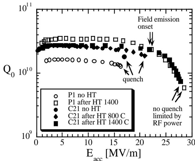
Fig. 2: Benefit of heat-treatment on cavities P1 and C21. After a heat-treatment of 1400 °C the maximum accelerating gradient in both cavities exceeded 28 MV/m. In the case of C21 it is shown that a 800 °C heat-treatment can also improve the RF performance, although the RRR does not change.
