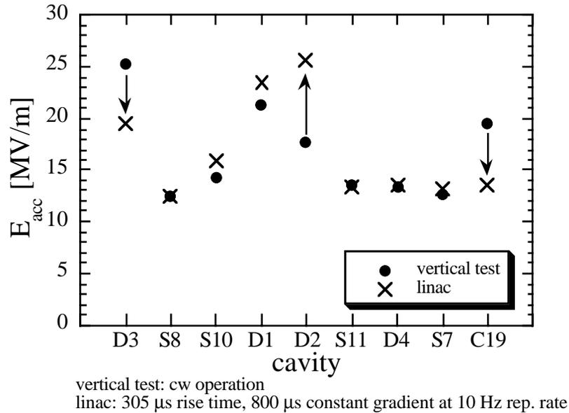
Fig. 8: Comparison of vertical test results to the performance of the cavities after installation in the linac. 2 cavities degraded caused by higher field emission loading, one cavity improved.
