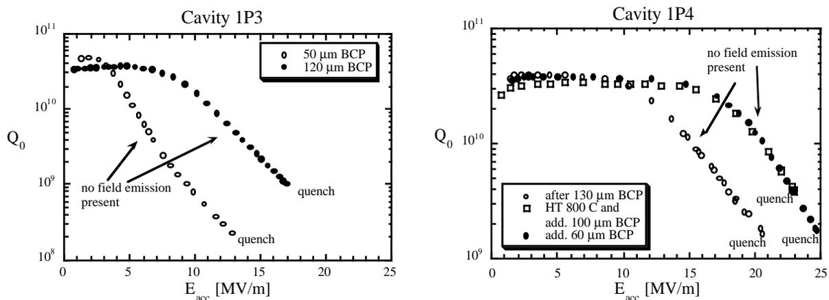
Fig. 6: RF performance of the first 1.3 GHz single-cell cavities made by spinning.
