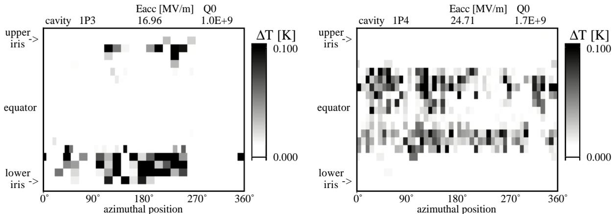
Fig. 7: Temperature maps of the single-cell cavities 1P3 and 1P4 at fields just below the quench. The maximum temperature rise was 400 mK in both cases. The temperature scale is set to 100 mK in order to display also areas with lower heating. The heating areas are causing the Q-drop at high gradients (see. Fig. 6).
