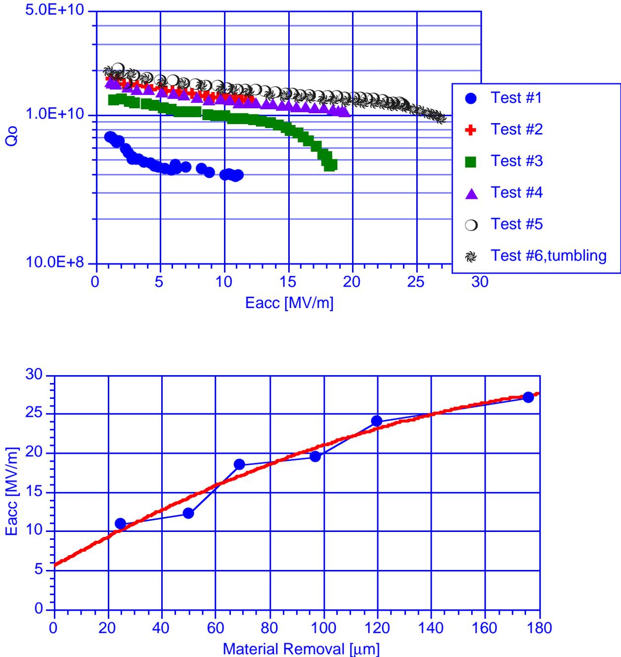
Figure 3: Performance of a 1300 MHz KEK-type single cell cavity (K-17) after subsequent amounts of material were removed from the surface. In test #6 the cavity was tumbled for 48 hrs prior to buffered chemical polishing.
