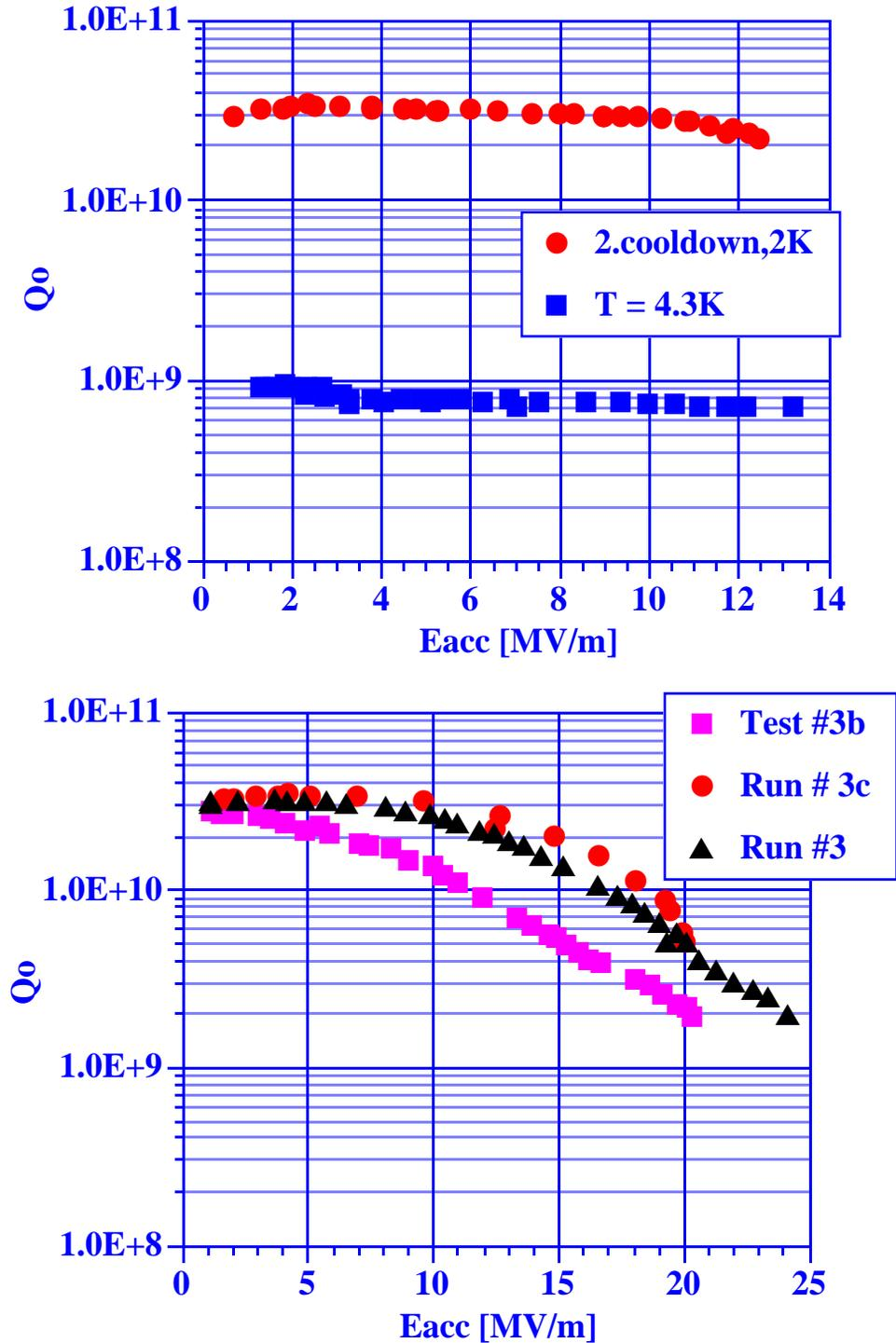
Figure 6: Performance of a sputtered niobium cavity prepared at CERN and tested at JLab after high pressure rinsing. Test 3b is after some quenches occurred in the cavity at higher gradients; test 3c was obtained after warm up to 100 K.
