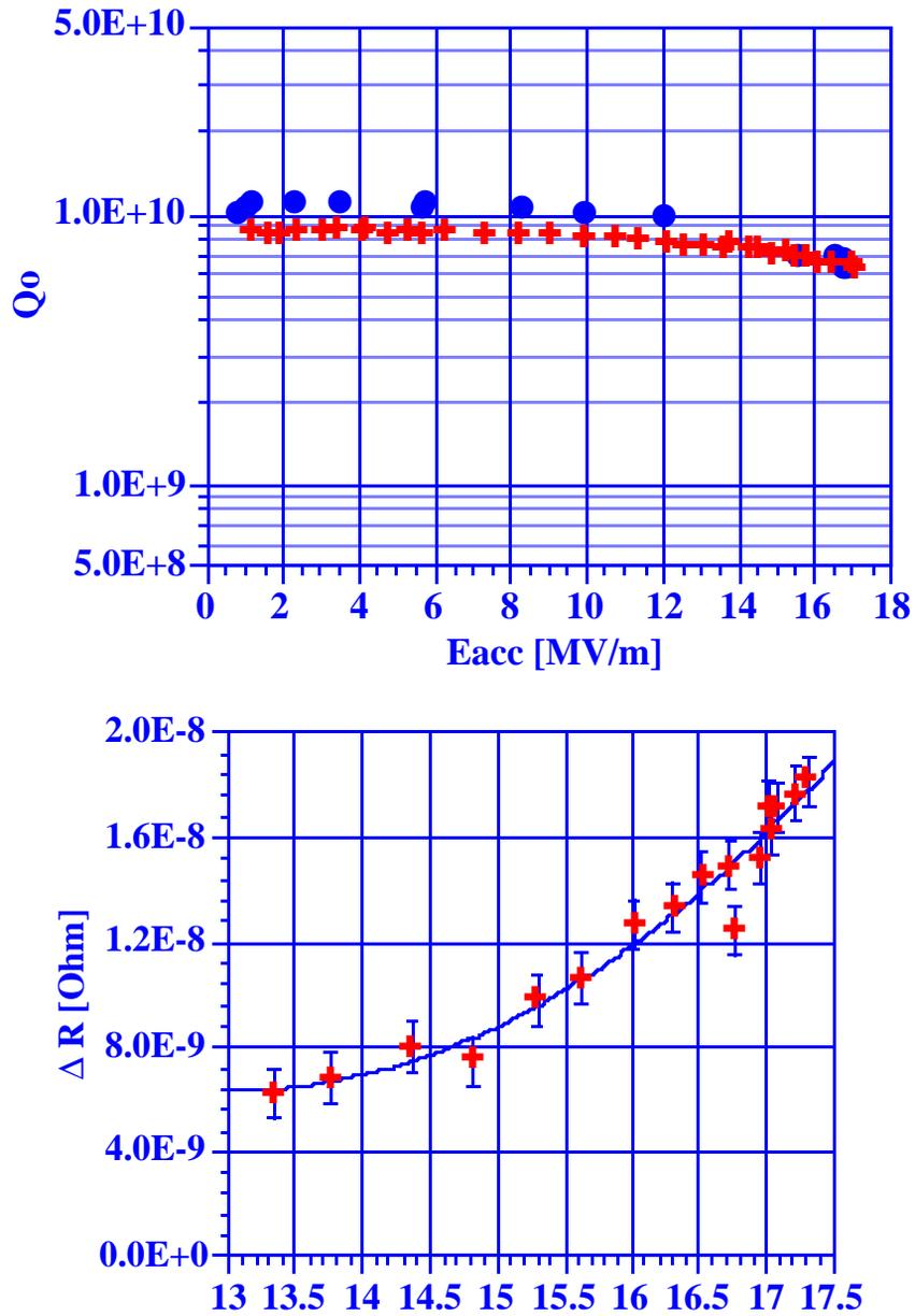
Figure 1 : Performance of "spare" cavity IA 363: Upper part shows  $Q_0$  vs  $E_{acc}$  , lower part shows the dependence of  $\Delta R$  on  $E_{acc}$  ( polynomial fit of 2nd order)
