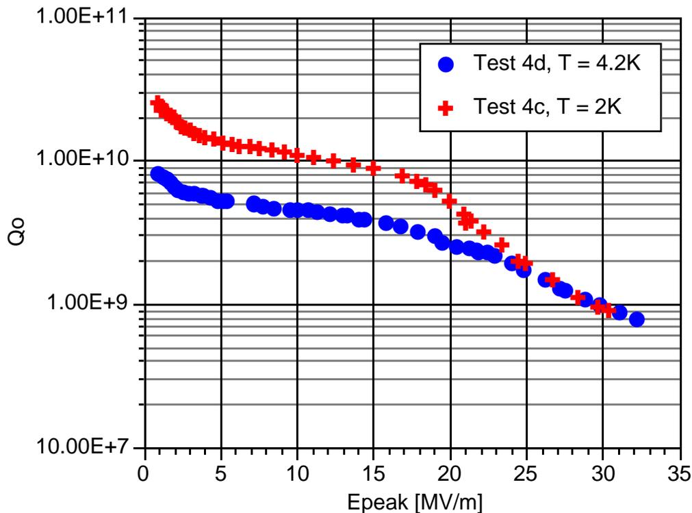
Figure 7:  $Q_0$  vs  $E_{\text{peak}}$  for the best Nb<sub>3</sub>Sn cavity prepared at the University of Wuppertal by the vapor diffusion process.
