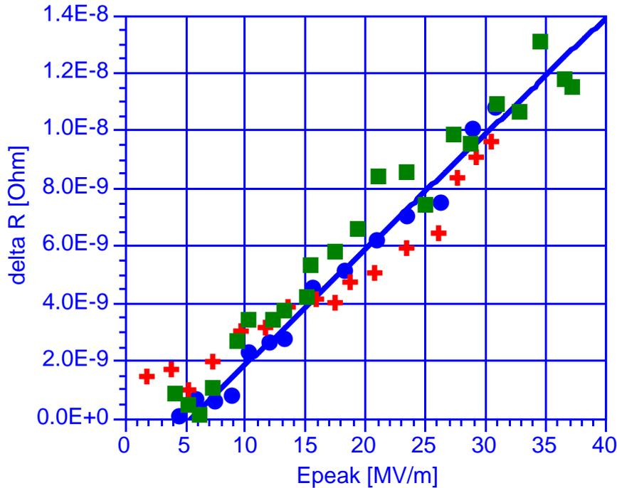
Figure 2: "TESLA Cavity" performance. In test #2a an emitter processed at  $E_p \approx 40$  MV/m, lowering the Q value in run 2b. The additional resistance causing the slope in  $Q_0$  vs  $E_{peak}$  is linear in  $E_{peak}$  as shown in the lower graph.
