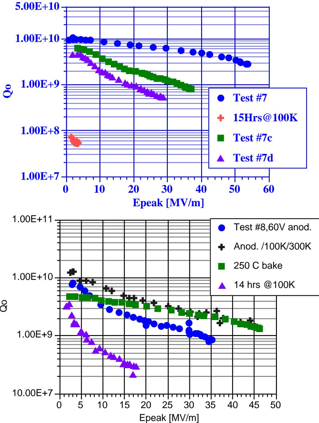
Figure 4: Results from the electro-chemical buffing surface treatment. Up to 300  $\mu\text{m}$  were removed from the surface by buffered chemical polishing. Q disease is shown in figure 4b, which did not even recover after warm-up to 300 K (tests 7c,7d). Figure 4c indicates some improvements in Q degradation after diffusion of oxygen into the surface layer.
