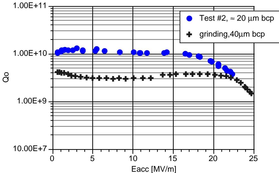
Figure 5: Performance of a seamless cavity fabricated by spinning, after heat treatment at  $1000^\circ \text{C}$  at CERN. The decrease in  $Q_0$  at high gradients (without observation of electron loading) is not clear.
