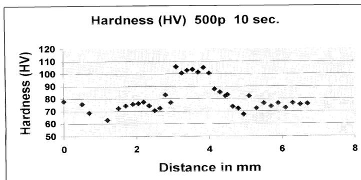
Fig. 9 Microhardness along the line through one of the Ta inclusions in the Ta test sheet
