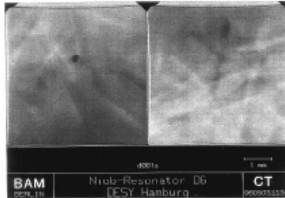
Fig. 2 Spot area of a dumb-bell of cavity D6
