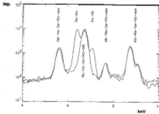
Fig. 13 Fluorescence spectrum of sheet T17, location 1
