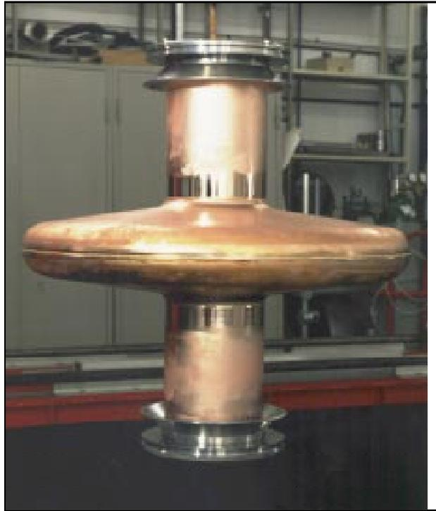
Photo: Copper cavity  $\beta=0.48$  ready for sputtering
