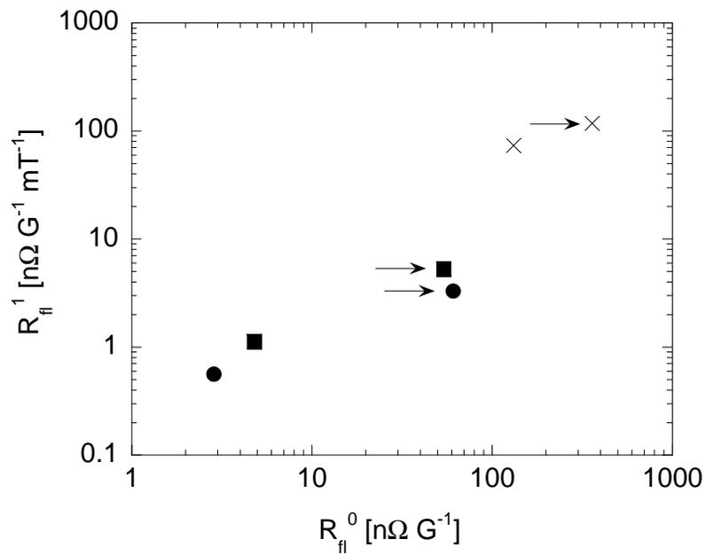
**Figure 7.** Effect of the change of sputter gas. Dots indicate krypton, squares argon and crosses neon. The arrows indicate cavities without the oxide interface.
