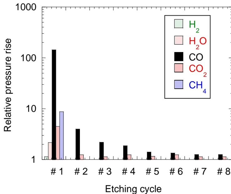
**Figure 3.** Relative pressure rise of the desorbed gases at each etching cycle.
