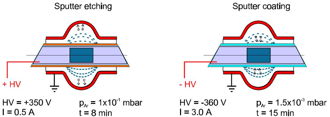
**Figure 2.** Sputter-etching and sputter-coating. The parameters used for the two discharges are also listed.
