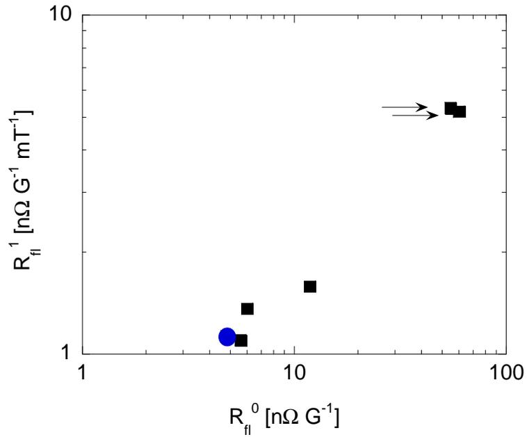
**Figure 6.** Effect of trapped magnetic flux on cavities coated using argon. Cavities without oxide interface are indicated by arrows. The average of 28 standard cavities is indicated by the dot, the error bars being smaller than it.
