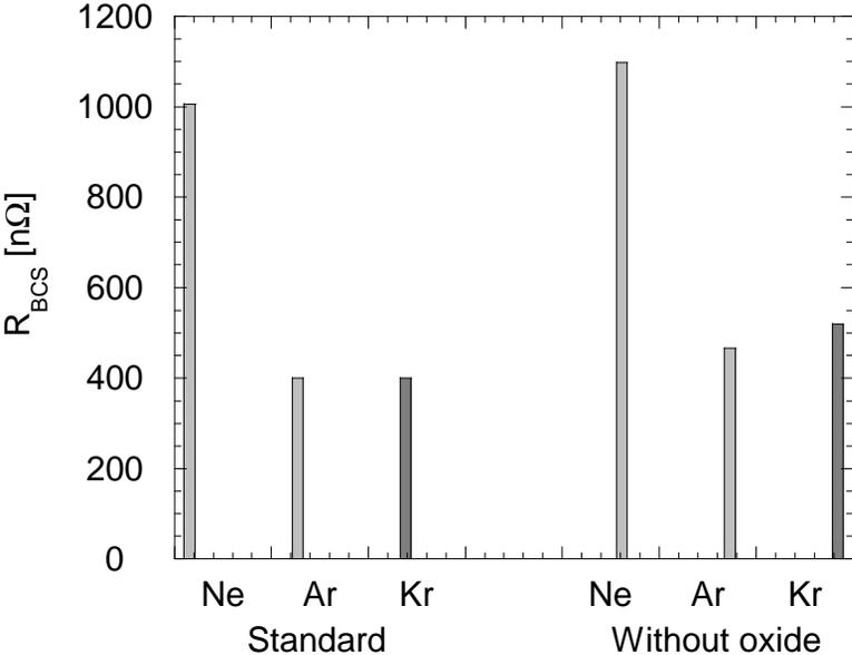
**Figure 5.**  $R_{BCS}$  for different discharge gases, with and without an oxide layer between copper and niobium
