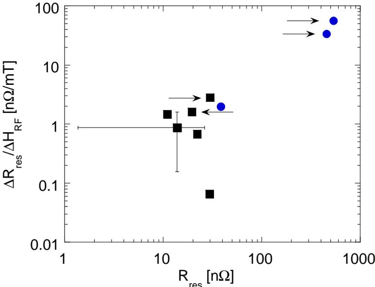
**Figure 4.** Residual resistance and its slope. Hydroformed cavities are indicated by dots, spun cavities by squares. The arrows indicate cavities that underwent sputter-etching as described in the text, compared to cavities with oxidation of copper after sputter-etching. The average of 28 cavities coated according to the standard procedure is also indicated with the error bars.
