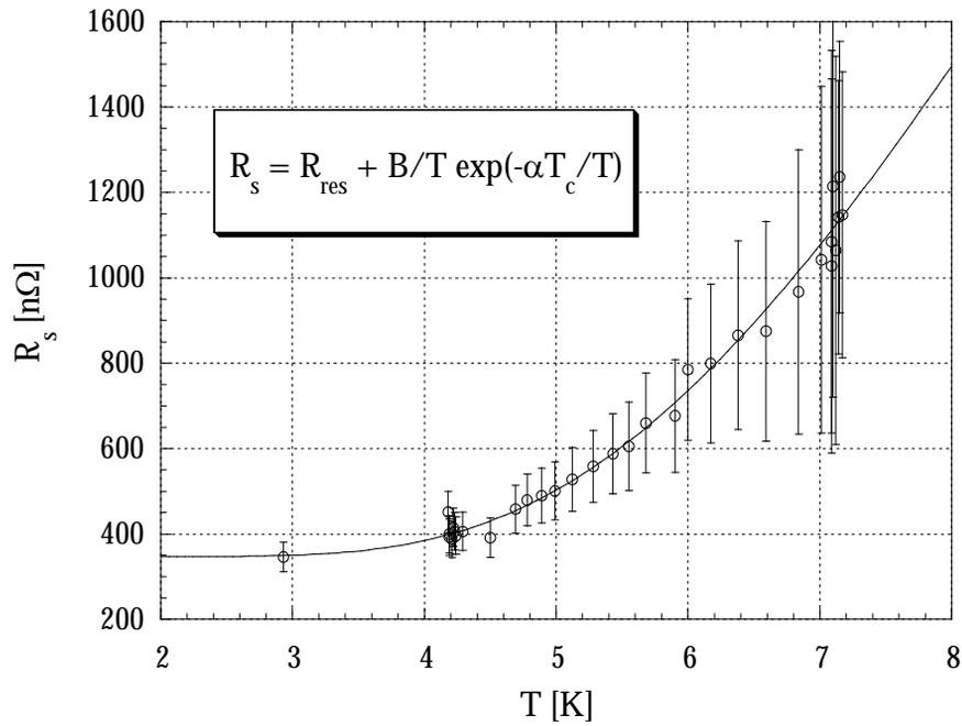
Fig. 6: Variation of the surface resistance as a function of temperature for  $H_{rf} = 0.23$  mT. From the displayed fit, putting  $T_c = 14.2$  K, one gets  $R_{res} = 350$  nΩ and  $\alpha = 2.3$ .
