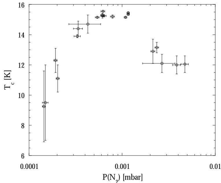
Fig. 2:  $T_c$  obtained on quartz samples as a function of the  $N_2$  partial pressure inside the cell during the coating. Data refer to the sputtering configuration shown in Fig. 1 and the discharge parameters indicated in the text.
