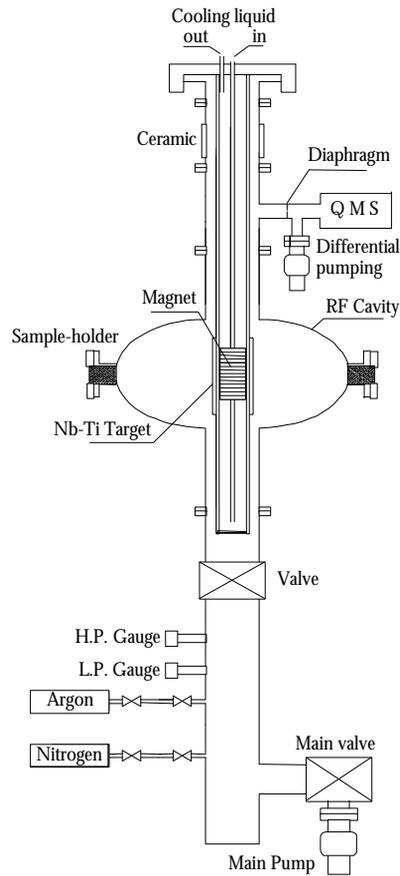
Fig.1: The sputtering system for the deposition of NbTiN thin films inside 1.5 GHz resonators.
