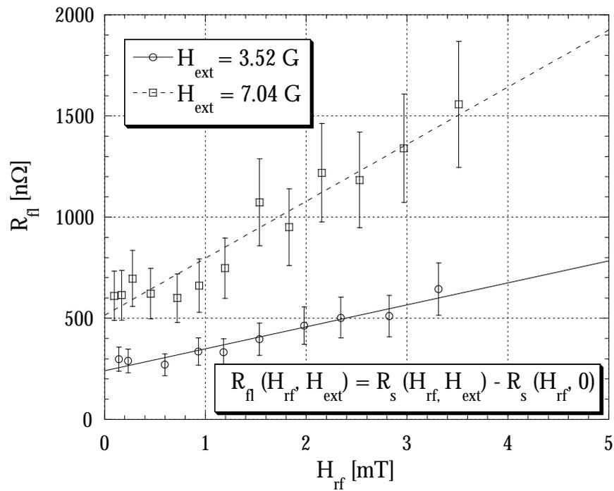
Fig. 7: Variation of the contribution induced by  $H_{ext}$  to the surface resistance of the resonator, as a function of the RF field  $H_{rf}$  for  $T = 4.2$  K. The displayed fit is of the form:  $R_{fl} = (H_{ext} - H_{th})(R_{fl}^0 + R_{fl}^1 H_{rf})$ .
