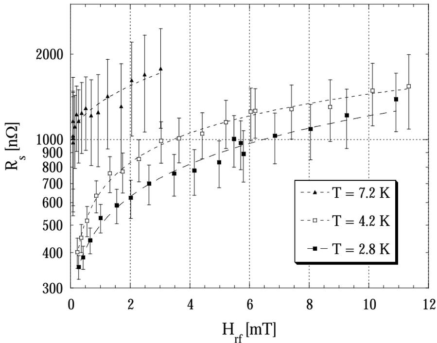
Fig. 5: Surface resistance of the 1.5 GHz NbTiN/Cu cavity as a function of the RF field at different temperatures.  $E_{\text{acc}} = 1$  MV/m corresponds to  $H_{\text{rf}} = 4.55$  mT.
