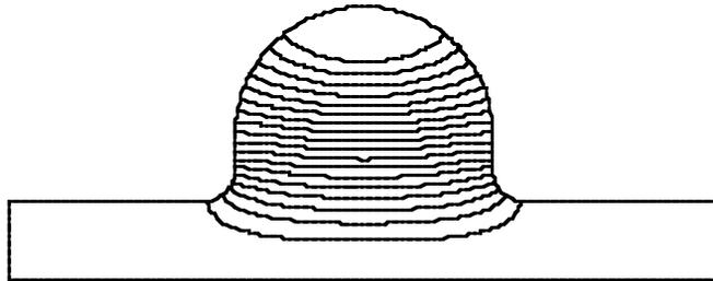
Fig 1; cavity shape with superimposed the electric field lines
