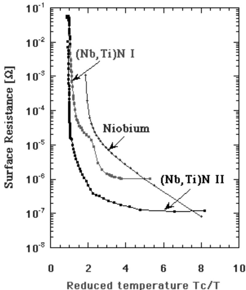
Fig 2; Surface resistance versus  $T_C/T$  for two cavities reacted for 6 hours (Nb-Ti)N I and 24 Hours ((Nb-Ti)N II. The theoretical BCS Surface resistance of the niobium is superimposed for comparison.
