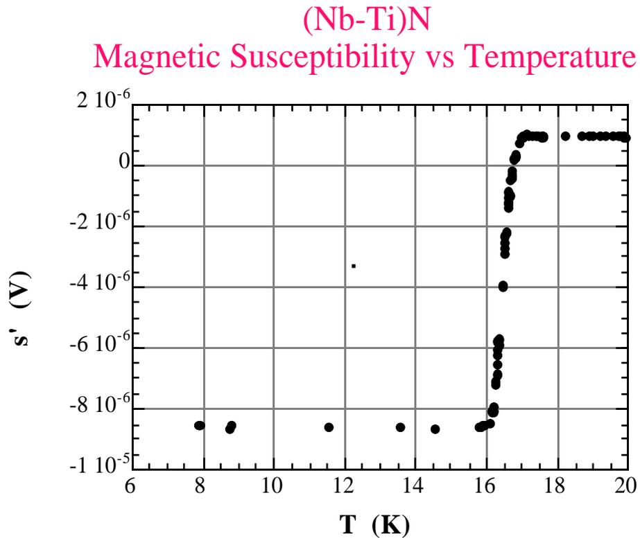
Fig. 5; AC susceptibility (real part) of a Nitride sample showing only a clean 17.2 K Tc phase on the sample surface.
