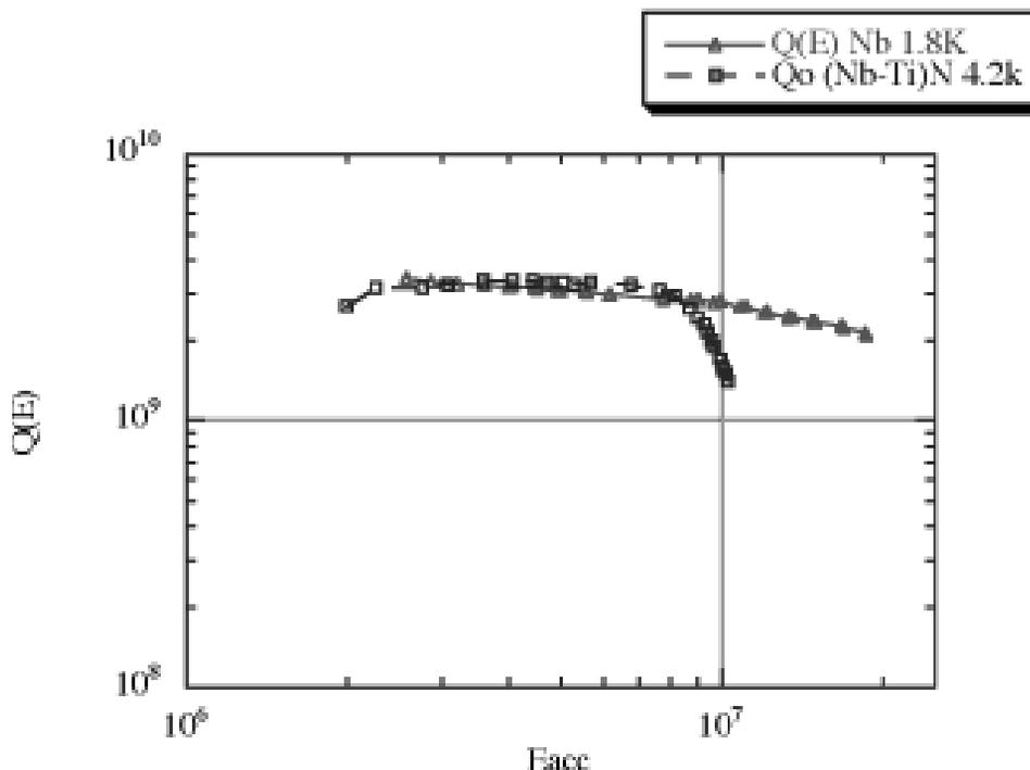
Fig 3; Quality factor versus accelerating field plot for the (Nb-Ti)N II cavity at 4.2K; the quality factor is constant as in a Niobium cavity at 1.8k till to the beginning of the NREL
