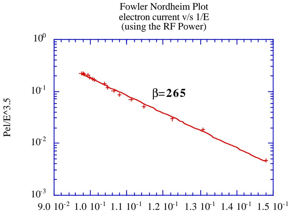
fig 4; Fowler-Nordheim Plot of the RF power dissipated by the electron current in the cavity showing a field enhancement of 265
