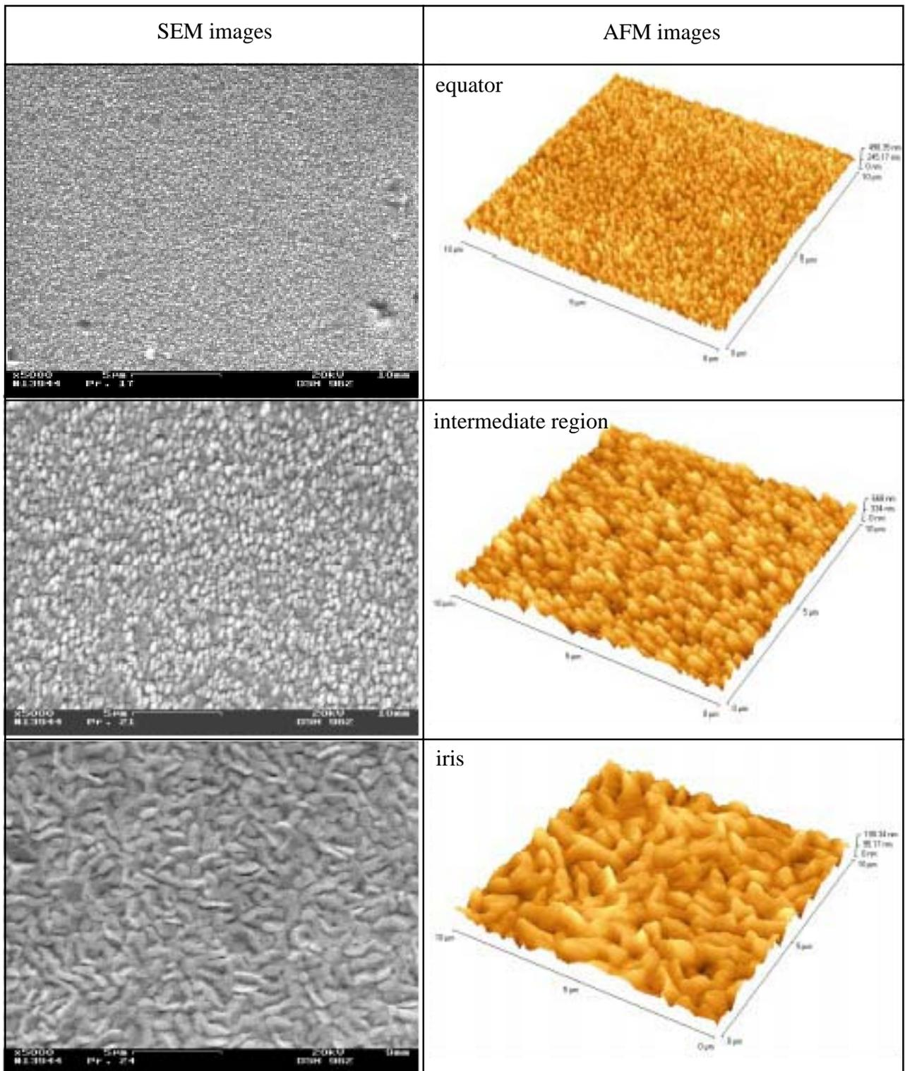
Fig. 2: SEM and AFM images of the Nb films on quartz substrates in dependence on the position in the 1.5 GHz resonator: equator, intermediate and iris regions
