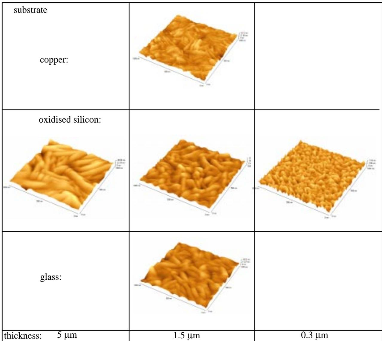
Fig. 3: AFM images of Nb films on different substrates and for several film thicknesses deposited by planar dc magnetron sputtering, each image:  $1\mu\text{m}^2$
