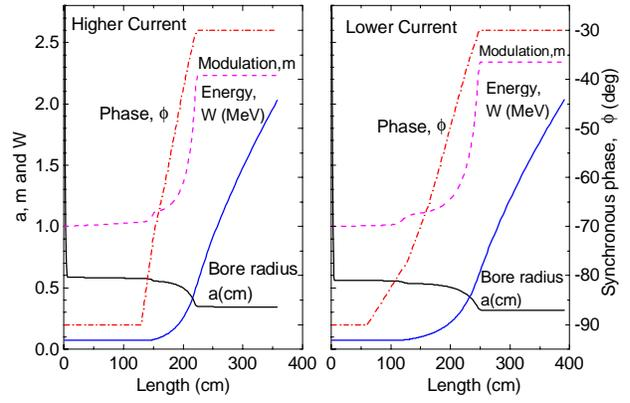
Figure 2. Design parameters for the higher and the lower current RFQs
