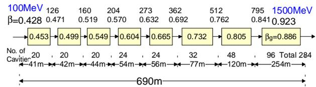
Figure 5. A schematic layout of the superconducting linac
