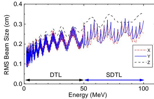
Figure 4. Beam sizes at the DTL and the SDTL
