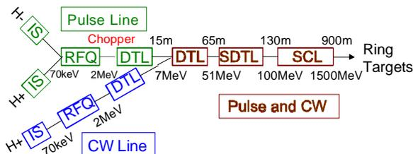
Figure 1. A schematic drawing of the linac system
