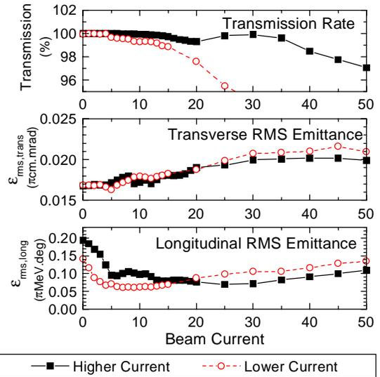
Figure 3. Transmission rate and normalized rms emittance for the higher and the lower current RFQs
