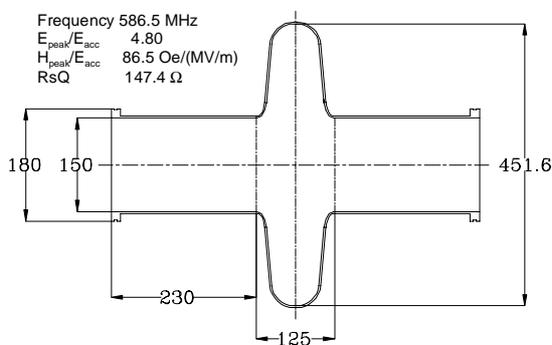
Fig. 1 Cross sectional view of the prototype single-cell cavity of  $\beta=0.5$
