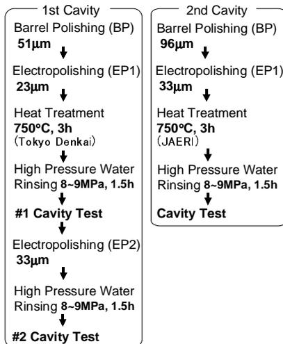
Fig. 2 Flow chart of the surface treatments and the performance tests
