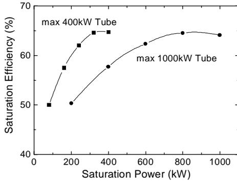
Fig. 4. Dependency of operating efficiency on saturation power. Beam voltage and anode voltage are controlled to saturate at a required power.
