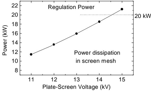
Fig. 2. Dependency of power dissipation on plate - screen voltage for 4CM2500KG.
