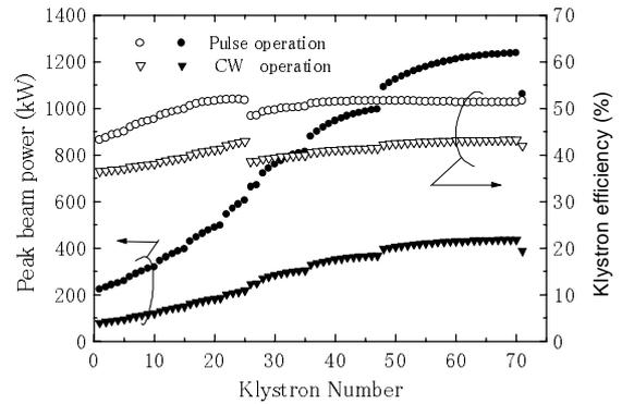
Fig. 5. Peak beam power and klystron efficiency for each klystron
