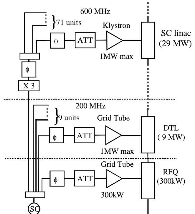
Fig 1. Block diagram of RF system for NSP accelerator.
