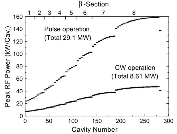
Fig. 3. Peak RF power for each cavity.
