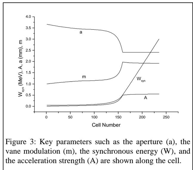
Figure 3: Key parameters such as the aperture (a), the vane modulation (m), the synchronous energy (W), and the acceleration strength (A) are shown along the cell.
