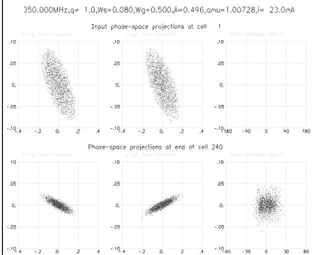
Figure 2: PARMTEQM simulation showing phase-space plots of the input beam and the beam at cell 240. The phase-space plots from left to right are:  $x-x'$ ,  $y-y'$ , and phase-energy, where  $x'=dx/dz$  and  $y'=dy/dz$ .
