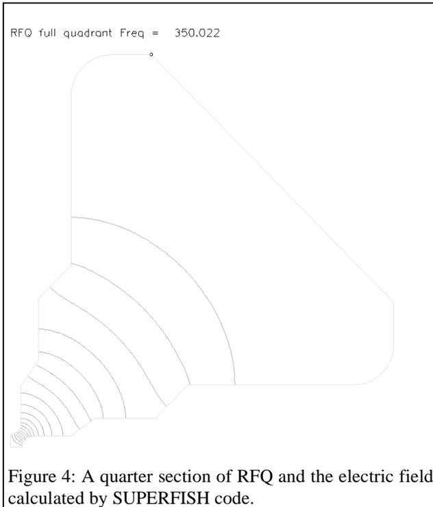
Figure 4: A quarter section of RFQ and the electric field calculated by SUPERFISH code.
