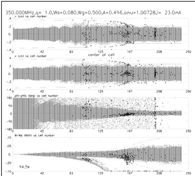
Figure 1: Results from PARMTEQM simulated the KOMAC RFQ using 5,000 particles. From top to bottom, the vertical axes are x, y, phase, and energy coordinates versus cell number, respectively. Bold black points indicate the lost particles. The transmission rate is 94.5%.
