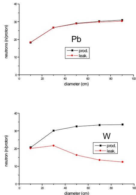
Figure 1: Neutron production and leakage as a function of target diameter (beam energy=1 GeV, height=50 cm).
