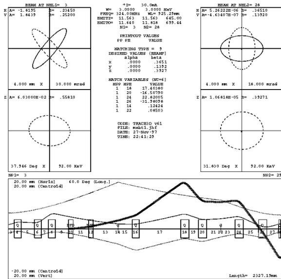
Fig. 1, TRACE3-D output of the MEBT for Type A. The up-left gives the input beam phase spaces and the up-right gives the matched beam with DTL. The bottom shows the beam profiles in z, x and y directions respectively. The dark line traces the beam centroid offset by the two RFDs. The element numbers are denoted under the beam axis.
