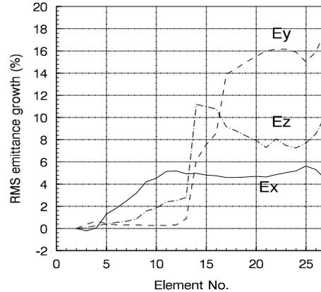
Fig.2. RMS emittance growth vs. the beam line elements for Type A
