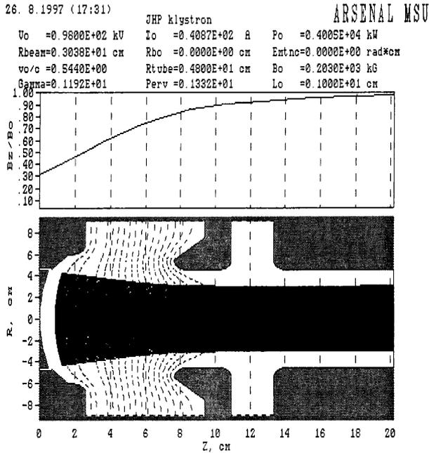
Figure 3: Modulation anode gun design of the klystron
