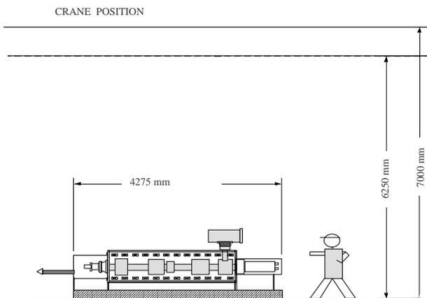
Figure 1: Horizontal mounting of the klystron
