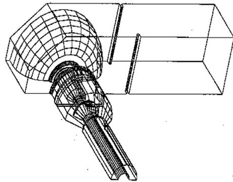
Figure 2: Window and coaxial-to-waveguide transition design of the klystron
