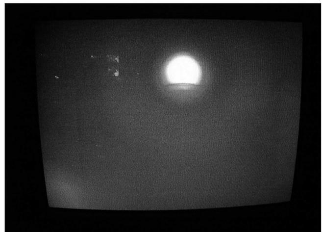
Figure 5: Glow light observed near to the inner conductor
