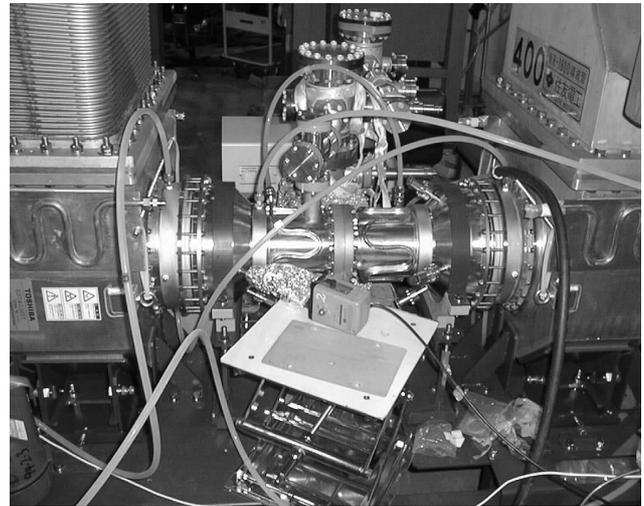
Figure 4: High power test of the co-axial window
