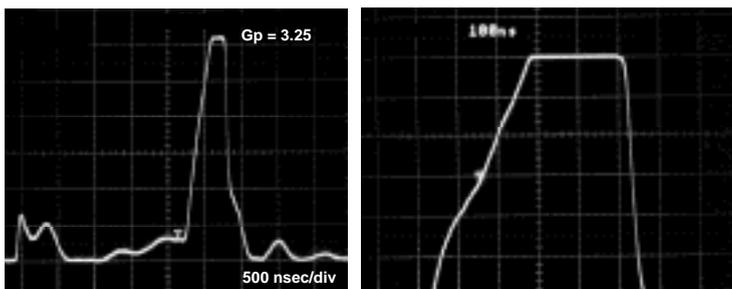
Fig. 3 Output pulse of C-band RF compressor and the magnified view of the flat top.
