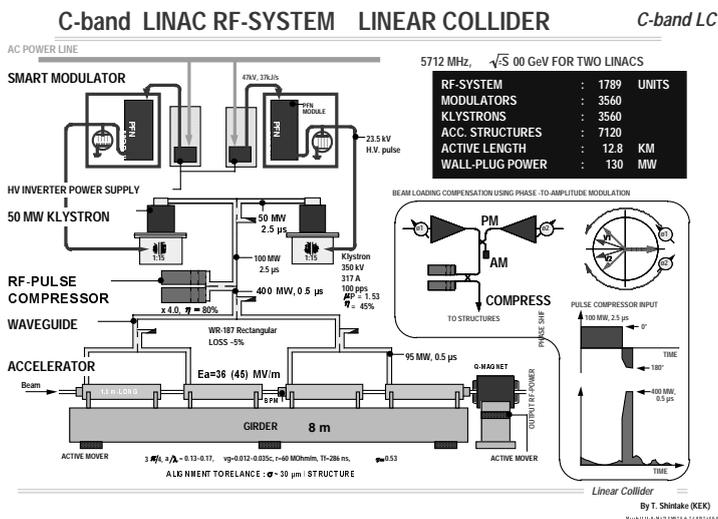
Fig. 1 One unit of the C-band RF system.
