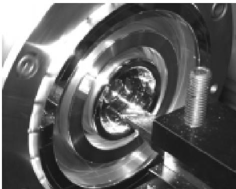
Fig. 7 A copper disk on a precision turning lathe. The main cavity part is machined with mirror surface using a diamond tip in order to maintain a high accelerating field. The choke-slot is sufficient with a standard machining. From center to outside: the beam hole, the main cavity, the choke-slot and a room for the HOM absorber (SiC ring).
