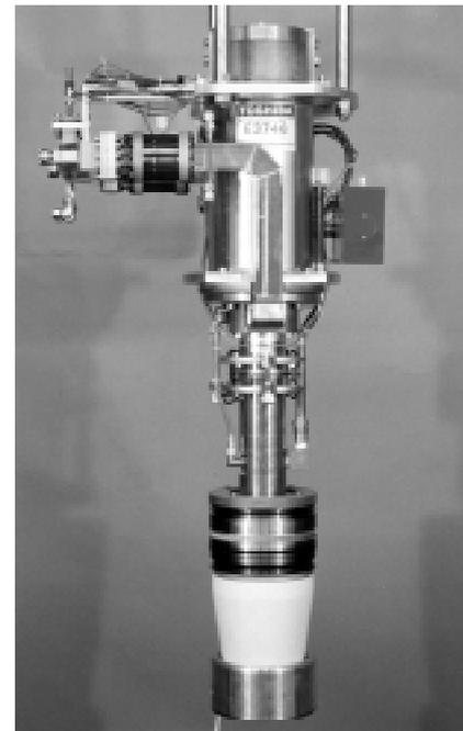
Fig. 4 The first high-power C-band klystron: TOSHIBA E3746 #1.
