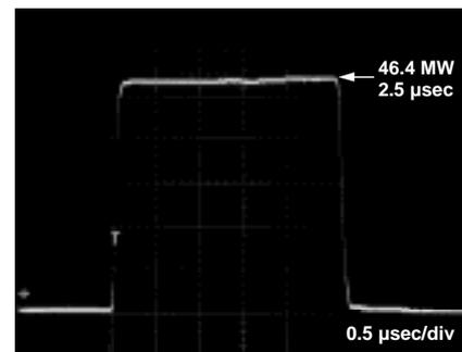
Fig. 5 RF output power from the first tube of E3746 C-band klystron.
