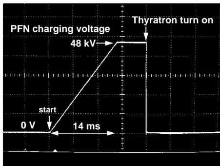
Figure 4 : Charging waveform of the PFN voltage. The external trigger starts the charging at 20 msec before the thyatron trigger (command charging).
