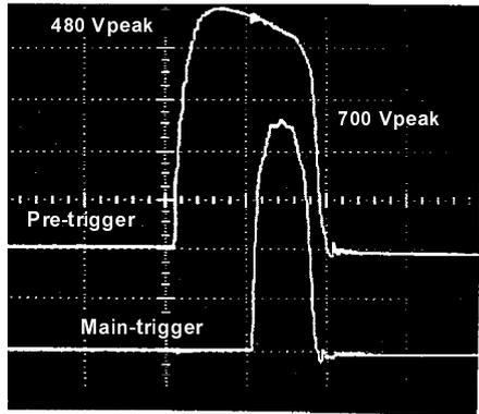
Figure 5 : Double-pulse thyatron trigger. The top waveform is the pre-ionizing pulse, and the bottom waveform is the main trigger to start discharge. Time scale is 1  $\mu$ sec/div.
