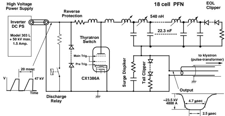
Figure 2 : Circuit diagram of the C-band klystron modulator.
