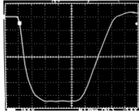
(a) Output voltage on the electron-gun of the C-band klystron. (350 kV peak, 1  $\mu$ sec/div)
