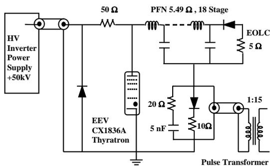
Figure 1. Circuit diagram of the C-band modulator
