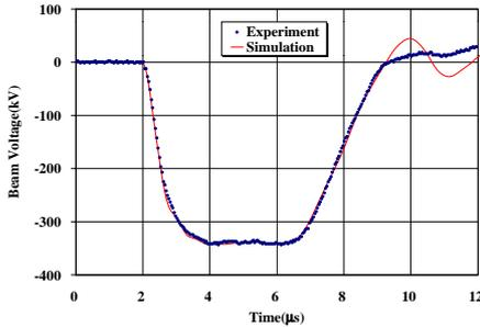
Figure 4. Pulse waveform of klystron beam voltage.
