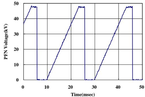
Figure 2. Charging waveform of the PFN.
