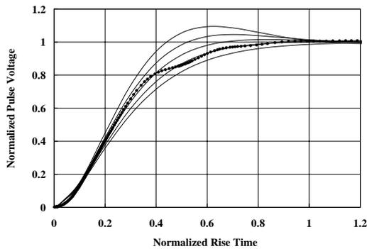
Figure 6. Analytic rising curves and beam voltage trace.
