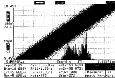
Figure 5. Jitter distribution of the beam pulse.
