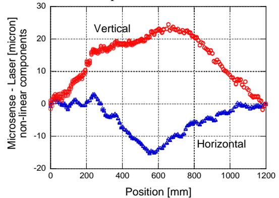
Figure: 6 Alignment measurement after diffusion bonding. Five successive measurements were superimposed.
