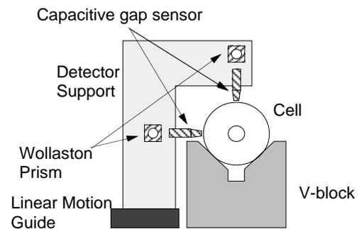
Figure: 3 Cells are stacked on a V-block. The alignment of the cells are measured using the capacitive sensor at top and side of a cell. The position of each capacitive sensor are calibrated by measuring the position of Wollaston prism located on the axis of the relevant sensor. The capacitive sensors and prisms are set on a single girder running parallel to the V-block guided by a linear-motion guide rail.
