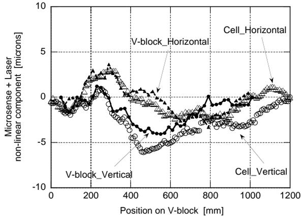
Figure: 4 Lines are the straightness of V-block. Open symbols are position of cells after stacked on it which is slanted at 60 deg.
