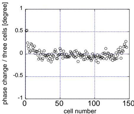
Figure: 2 Bead pull measurement for the same structure as the previous figure.
