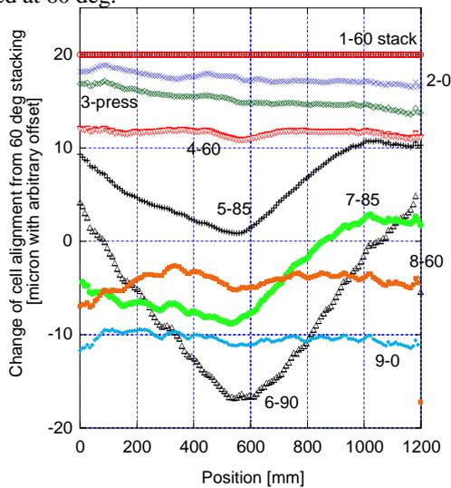
Figure: 5 Change of cell alignment due to rotation of the stacked cell from horizontal towards vertical position. First numbers are the order in the study and the second number following hyphen are the angle of the V-block.
