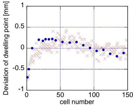
Figure: 1 Deviation of dwelling point from the mechanical center of cells for a detuned structure.
