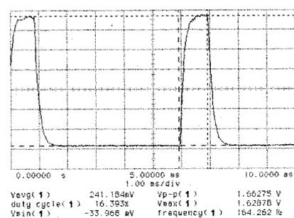
Fig.6 The  $O^+$  pulse beam at RFQ entrance
