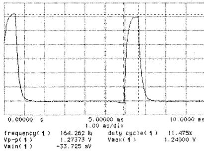
Fig. 8 The output beam wave form when 70% injected  $O^+$  beam is put in rf pulse and accelerated
