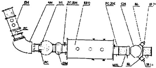
Fig. 4 Layout of the ISR RFQ Accelerator
