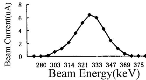
Fig.5  $N^+$  energy spectrum at 45kW
