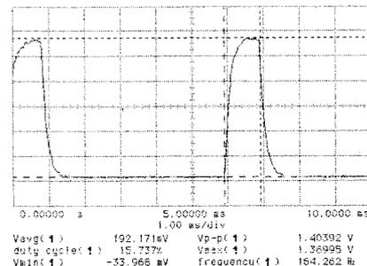
Fig.7 The  $O^+$  pulse beam at RFQ exit
