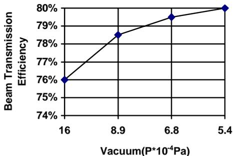
Fig. 11 Beam Transmission via Vacuum status
