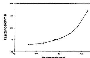
Fig.3 The input impedance of 300keV ISR RFQ
