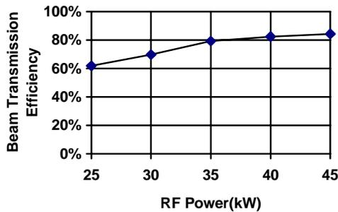
10 Beam Transmission via RF Power
