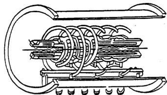
Fig.1, The Structure of 300keV ISR RFQ
