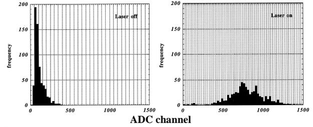
Fig.4 Collision frequencies measured with air Cerenkov counters for laser-on and laser-off.
