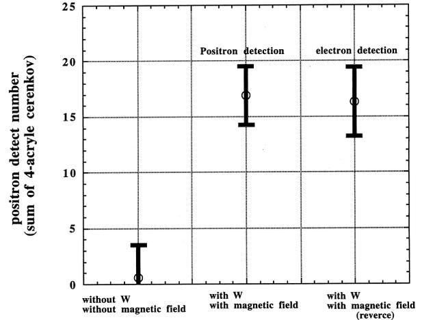
Fig. 6 Numbers of  $e^+$  / pulse detected under the conditions : (a) Without a W-target and magnetic field, (b) With a W-target and magnetic field, (c) With a W-target and magnetic field (reversed current)
