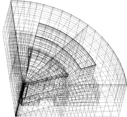
Fig.3 3D Mesh of the Magnet (1/8)
