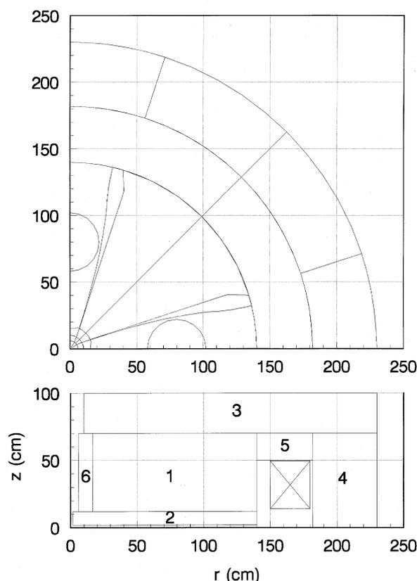
Fig. 1 The Geometry of CYCIAE-70 Magnet
