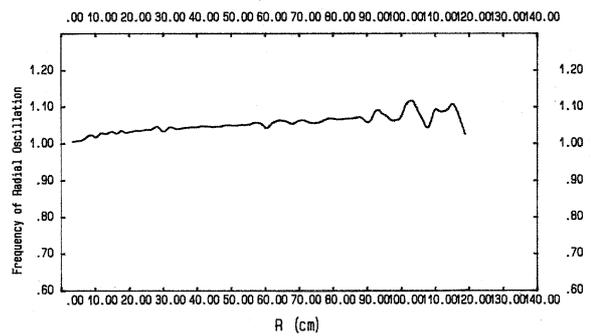
Fig.8 (b) The Frequency of Betatron Oscillation (radial oscillation)
