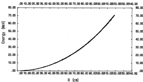
Fig. 7 The Extraction Position of Different Energy
