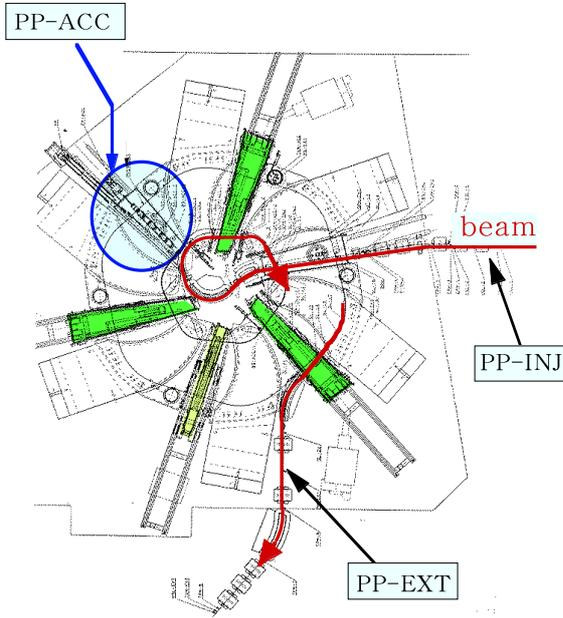
Figure 1: **Top view of the Ring Cyclotron** The 8 capacitive detectors are installed in the circled area. These detectors are named as 'Probe-Channel 1...8' from the inside of the orbital radius. These plates are  $45 \times 45 \text{ mm}^2$  or  $30 \times 65 \text{ mm}^2$  in size and  $35 \text{ mm}$  in distance between upper and lower plates.
