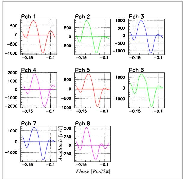
Figure 6: Beam-response input waveform to the sampling circuit It is reconstructed by the fourier information until the 60th harmonic components. The probe-channel is indicated by 'Pch'.
