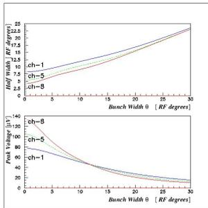
Figure 3: **Simulation result** The X-axis of both figures are the beam-bunch half width of a circulating beam. The upper figure is beam-response half width correlation, the lower figure is beam-response peak voltage one.
