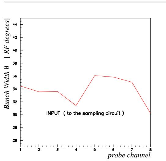
Figure 7: Transition of the circulating beam-bunch half width
