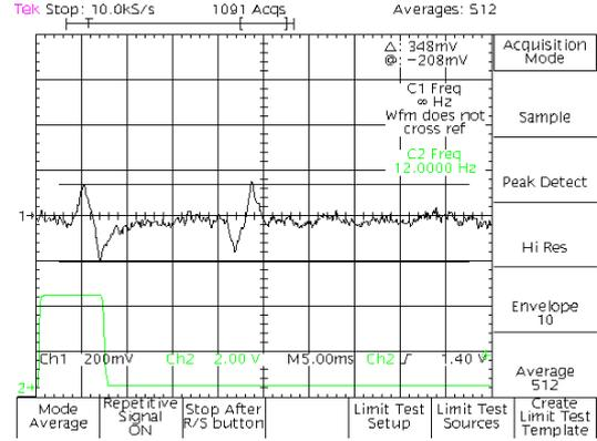
Figure 4: **Final-output** The extraction beam current is 3nA, and the averaging is 512 times. Scope: 108 RFdegrees/div, 200mV/div
