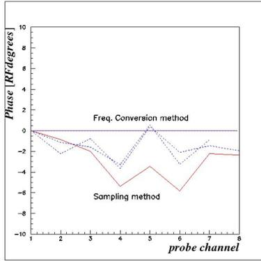
Figure 5: Phase difference between the frequency conversion and the sampling method
