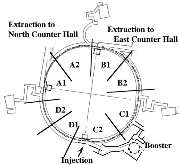
Figure 3. Foundations of the Main Ring Floor, comprising eight separated plates.
