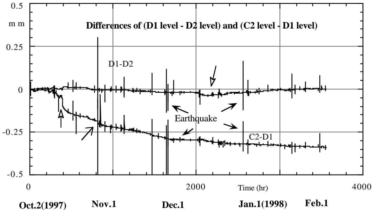
Figure 4. Time variation of the floor level differences of C2-D1, and that of D1 -D2. Floor level difference of C2-D1 changed rapidly (in fifty hours) by about 0.15 mm in the middle of October, 1997 and it increased gradually up to 0.35 mm for a few months. Many seismic vibrations were observed indicated by the dark arrows for example. At the end of October, as indicated by the simple arrow, the difference did not return to the one before earthquake.
