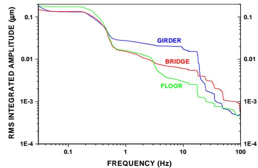
Figure 4: Horizontal vibration in the experimental hall of KEKB.
