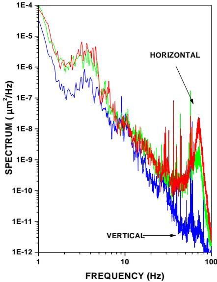
Figure 1: Ground motion in the quiet granite site.
