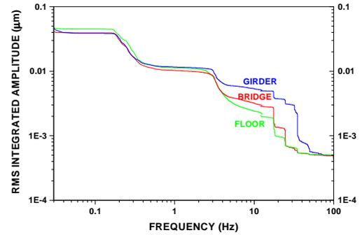
Figure 3: Integrated vertical vibration in the experimental hall of KEKB. BRIDGE is a construction on the floor and GIRDER is set up for the final focus magnet.
