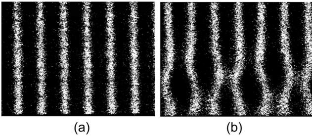
Fig. 1. Snapshots taken every 4  $\mu\text{sec}$  before and after the turn-off of the ion pumps. Total time span in horizontal direction is 25  $\mu\text{sec}$  (6.4 mm in spatial unit), and 500 nsec in vertical direction. a) Snapshots taken at nominal condition. Very weak oscillation was observed at the very tail of the bunch train. b) After ion pumps were turned off, the snake-tail oscillation at the tail is clear.
