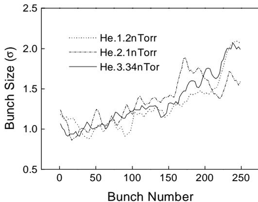
Fig. 4. Bunch size measured along the bunch train for three different cases of 1.2 nTorr, 2.1 nTorr, and 3.34 nTorr showing the same growth pattern. Bunch sizes are normalized to the initial bunch size.
