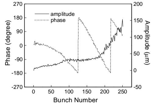
Fig. 3. The phase advance and amplitude of bunch train oscillation plotted from an SBPM data taken before the He injection. Phase advance per bunch is  $\sim 2\pi/95/\text{bunch}$  at the tail, which agrees with the frequency of 5.4 MHz measured with the spectrum analyzer
