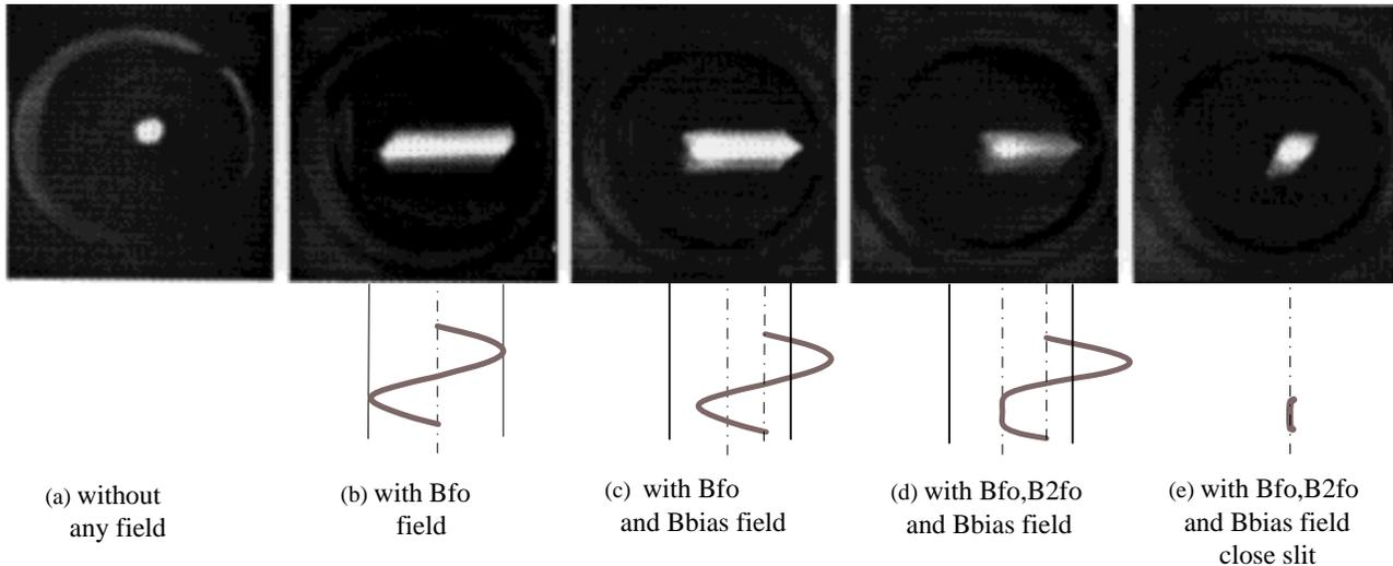
Fig.4 Beam profile change during the chopper system adjusting
