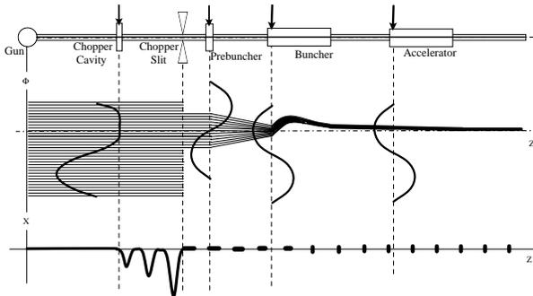
Fig.2 Beam and RF Phase Relationship in the Injector
