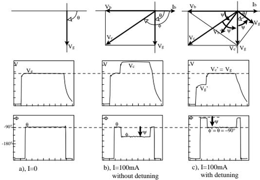
Fig.5 Prebuncher Cavity with Beam Loading and Cavity Detuning
