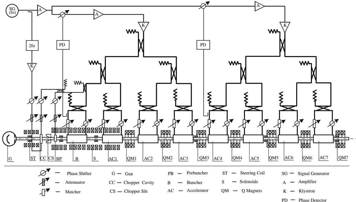
Fig.1, Schematic Layout of PNC High Power Linac
