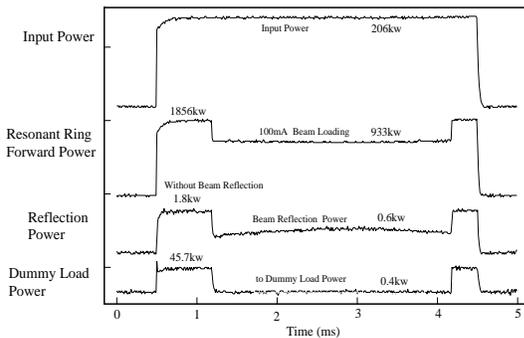
Fig.6 RF Waveform under beam loading in accelerator section
