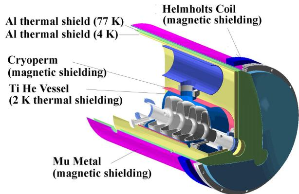
Figure : 5 Conceptual layout of magnetic and thermal shielding
