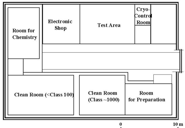
Figure : 6 Layout of KOMAC SC cavity R&D facility
