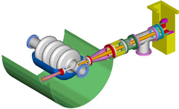
Figure : 4 Conceptual layout of KOMAC input coupler
