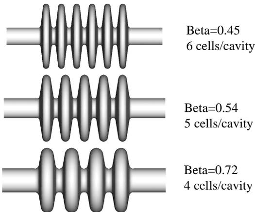
Figure : 3 The optimized cavity shapes for each beta
