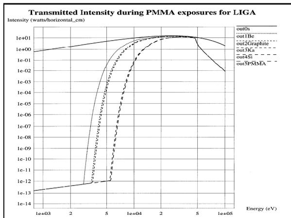
Figure 2: Transmitted x-ray intensity during PMMA exposures for DXRL at APS, energy vs. intensity.
