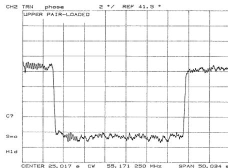
Fig.6- Results of the Phase Shift Method
