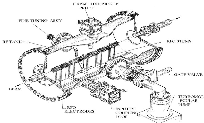
Fig.1-Isometric View of LPRFQ Accelerator
