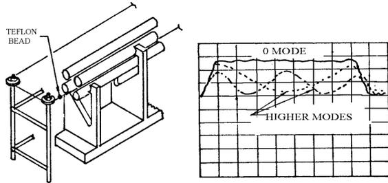
Fig.2-Bead Perturbation Assembly Fig.3- Electric Field Distribution of various modes
