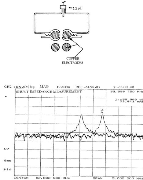
Fig.5- Setup and Results of Frequency Shift Method for the Measurement of Shunt Impedance MHz.
