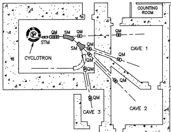
Figure 3: Layout of the beam lines for the superconducting cyclotron planned in the first phase at VECC
