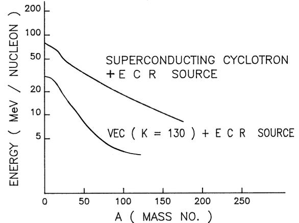
Figure 1: Energy/nucleon vs. mass for heavy ion beams to be available with VEC and superconducting cyclotron
