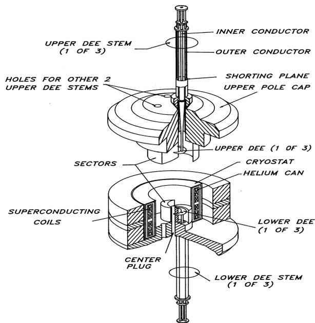
Figure 2 : Cross sectional view of the superconducting cyclotron at VECC
